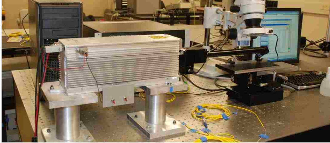
Figure 6.2 Photo of CO 2 laser irradiation system
