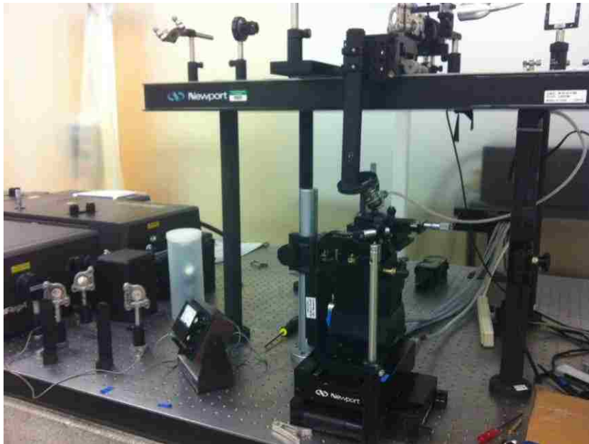
Figure 3.1 Photo of femtosecond laser micromachining system
