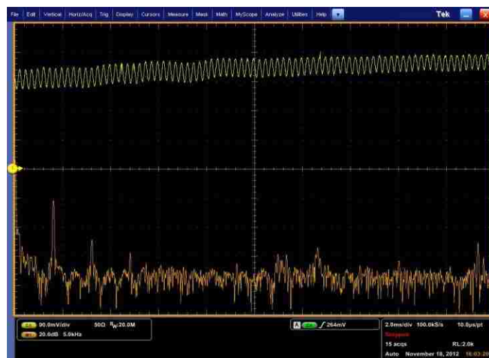
Figure 5.4 Acoustic response to 4 kHz sinusoidal signal
