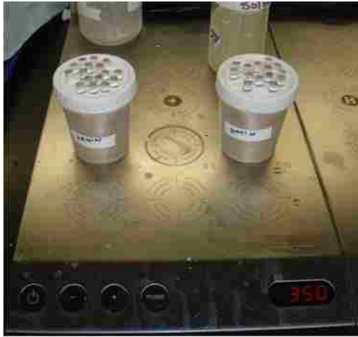
FIGURE 7. Enamel specimens mounted on plastic rods and submerged in 50/50 saliva in the remineralization/demineralization pH cycling model.
