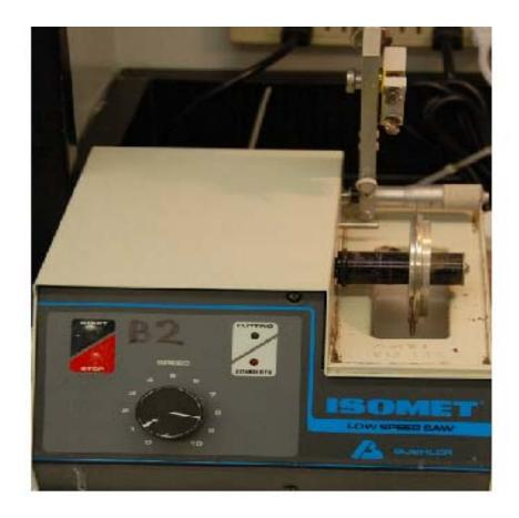
FIGURE 10. Image of Buehler Isomet low-speed saw.
