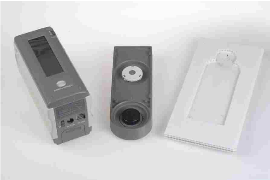
Left to Right: a) Spectrophotometer b) calibration plate c) Jig with a white background
