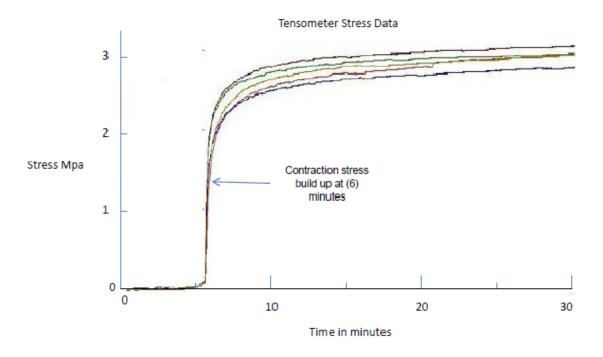
FIGURE 8. Graph showing contraction stress (MPa) of the 6-min delayed-cure group (Group D).
