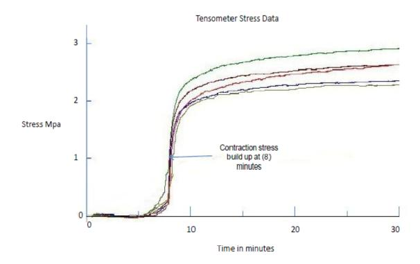
FIGURE 9. Graph showing contraction stress (MPa) of the 8-min delayed-cure group (Group E).
