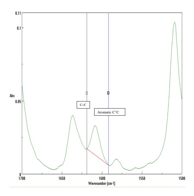
FIGURE 4. Graph showing ATR spectra of uncured luting resin.
