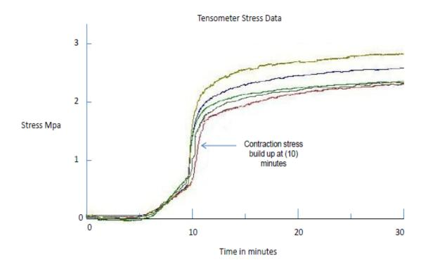
FIGURE 10. Graph showing contraction stress (MPa) of the 10-min delayed-cure group (Group F).
