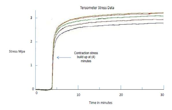
FIGURE 7. Graph showing contraction stress (MPa) of the 4-min delayed-cure group (Group C).
