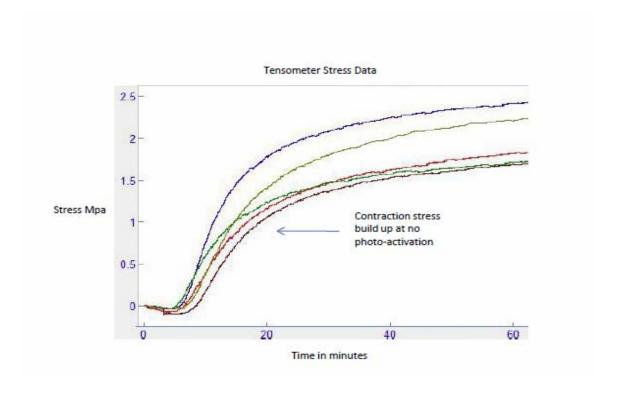
FIGURE 11. Graph showing contraction stress (MPa) of the group receiving no photo-activation (Group G).
