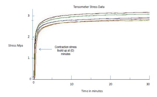
FIGURE 5. Graph showing contraction stress (MPa) of the immediate light-cured group (Group A).
