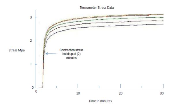
FIGURE 6. Graph showing contraction stress (MPa) of the 2-min delayed-cure group (Group B).
