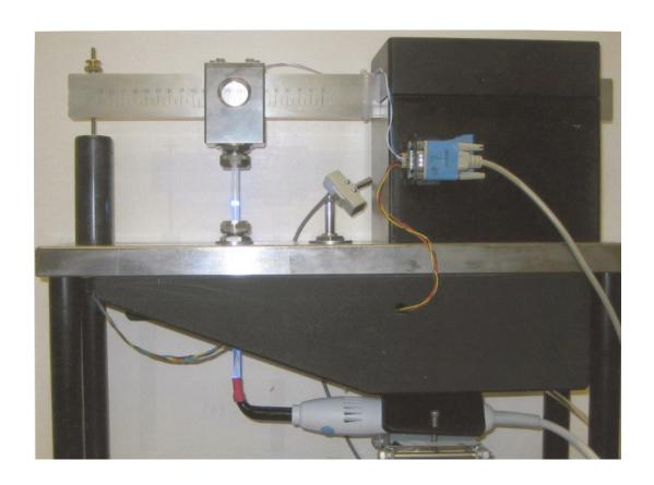
FIGURE 1. The ADA tensometer.
