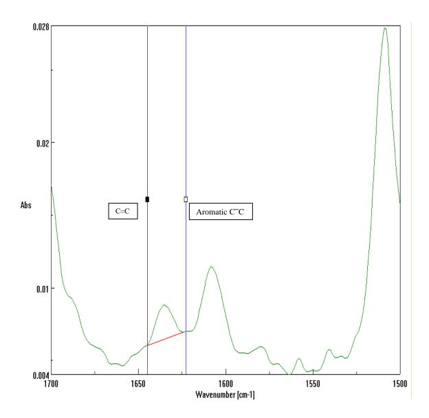
FIGURE 3. Graph showing ATR spectra of light-activated luting resin.
