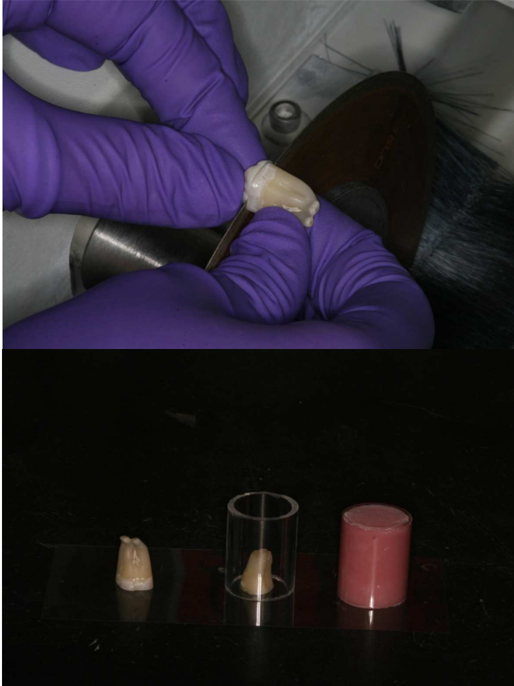
FIGURE 3: Molar preparation: Top – removal of cusps and occlusal enamel; Bottom – sequence of steps for mounting molars in acrylic resin.
