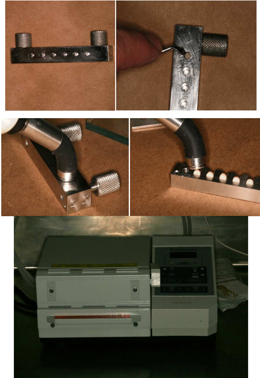
FIGURE 4: Indirect resin cylinder fabrication: Top Left – stainless steel split mold; Top Right – resin placement into mold; Middle Left – initial photopolymerization; Middle Right – additional polymerization; Bottom – Premise Indirect HP curing unit for final polymerization.
