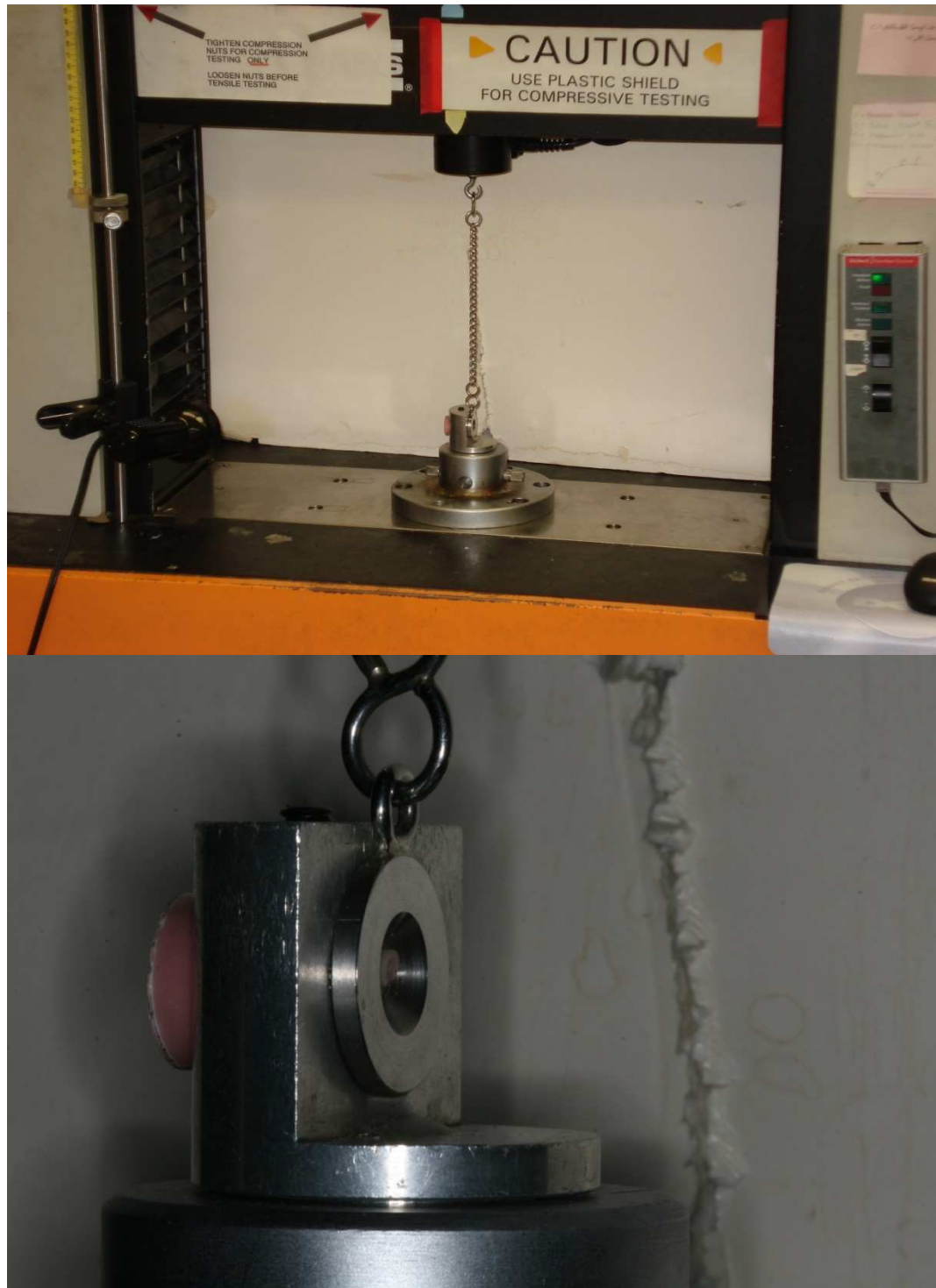
FIGURE 6: Top – shear bond strength/knife-edge shear testing apparatus on MTS machine; Bottom – close view of apparatus.
