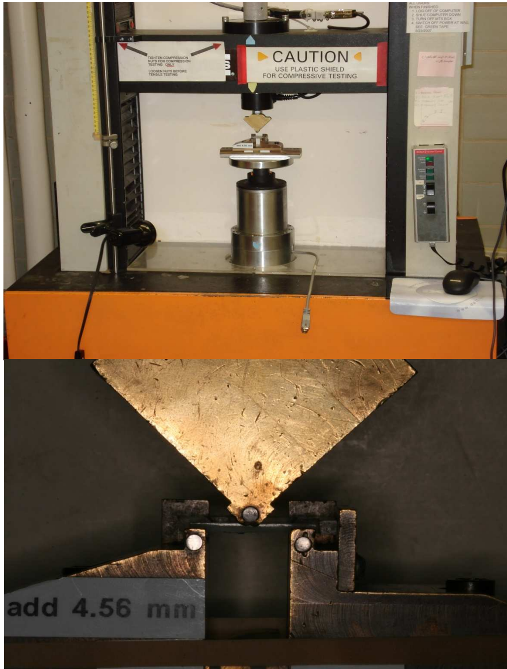
FIGURE 2: Top – flexural strength/three-point-bending testing apparatus on MTS machine; Bottom – close view of apparatus.
