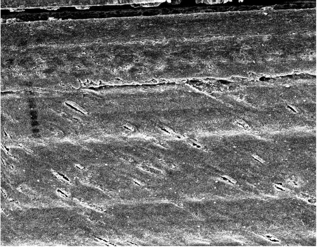
FIGURE 16. The SEM image of the control group of Variolink II. The separation was found between the adhesive layer and the resin composite (X500).
