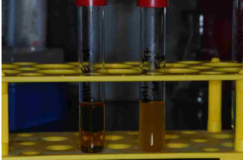
FIGURE 22. One day after broth inoculated with E. faecalis GFP. Sterile BHI-YE broth with tetracycline (left) and turbid broth displaying growth of E. faecalis GFP (right).
