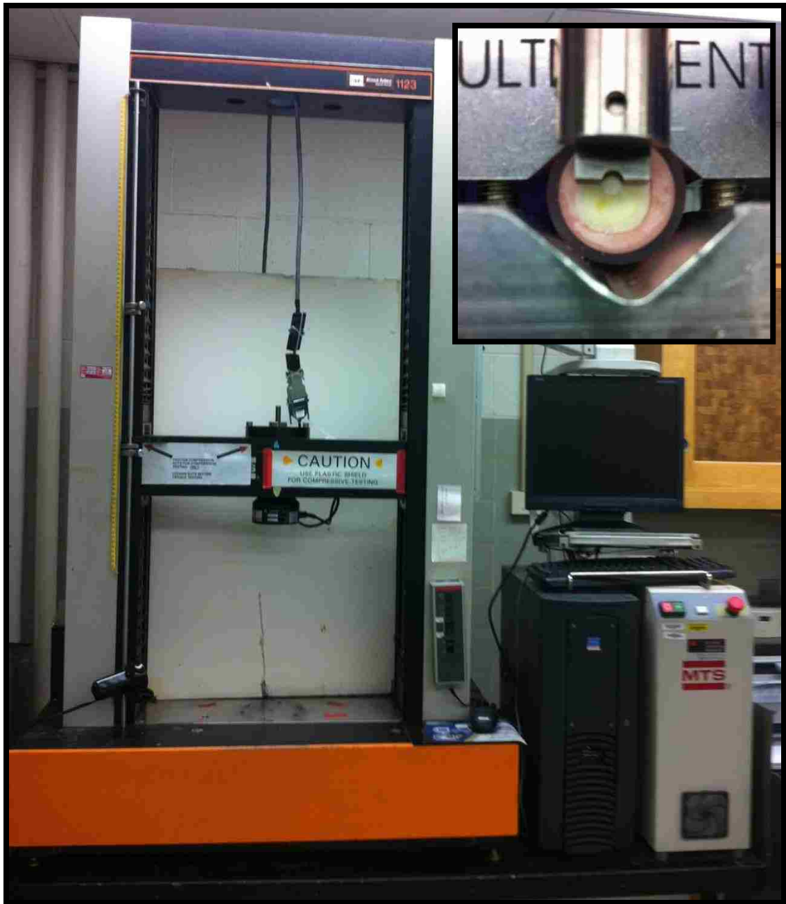
FIGURE 5. A. Universal testing machine (MTS Sintech Renew 1123, Eden Prairie, MN). B. Notched, semi-circular shaped edge (Ultradent Inc.).
