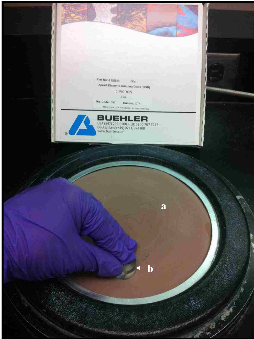
FIGURE 10. A. Apex ® Diamond Grinding Discs DGD, Buehler Ltd, USA. B. Specimen with resin bonded interface against the polishing disc.
