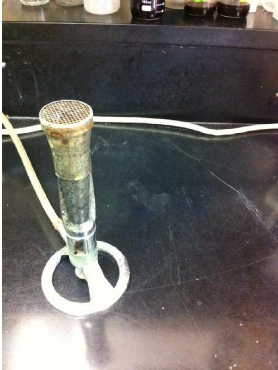
FIGURE 9. All pipette work performed adjacent to Bunsen burner on bench top to minimize bacterial contamination; also used to flame cervical area of containers prior to removing solutions with pipette.
