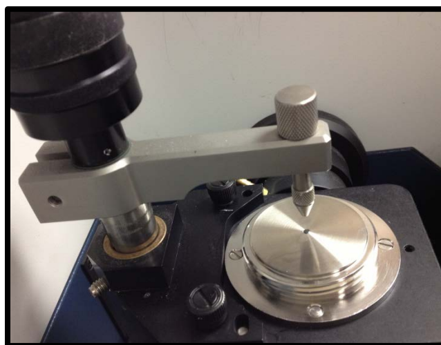
Figure 8: FTIR. Instrument (top) used to measure the degree of conversion. The ZnSe crystal and mounting assembly for such measurements (bottom).
