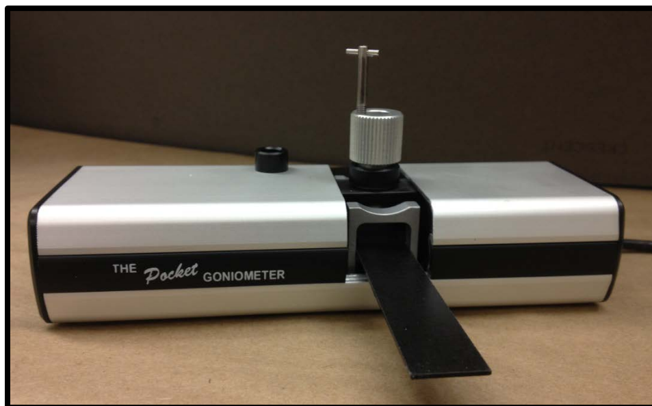
Figure 7: PocketGoniometer. Instrument used to image the side profiles of the cured resin bullets.
