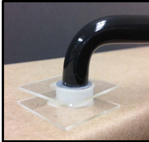
Figure 4: Experimental setup to investigate point light source curing. Arrangement of the glass slides, resin filled mold, and single aperture mask.
