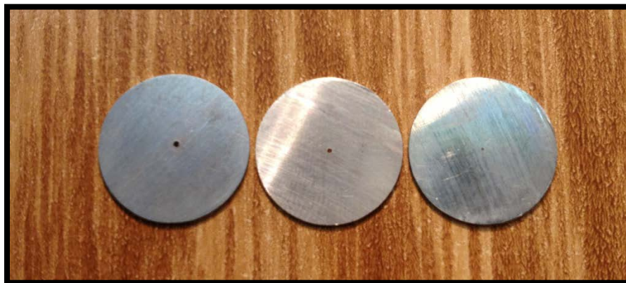
Figure 2: Single aperture masks. Left to right, the aperture diameters are 0.5 mm, 0.4 mm, and 0.25 mm respectively.
