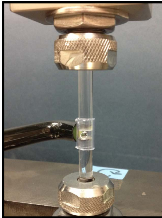
Figure 11: ADA tensometer. Instrument (top) for the measurement of polymerization shrinkage stress. The side curing approach testing setup for this study (bottom) with quartz rods, plastic tube, and curing light in position.
