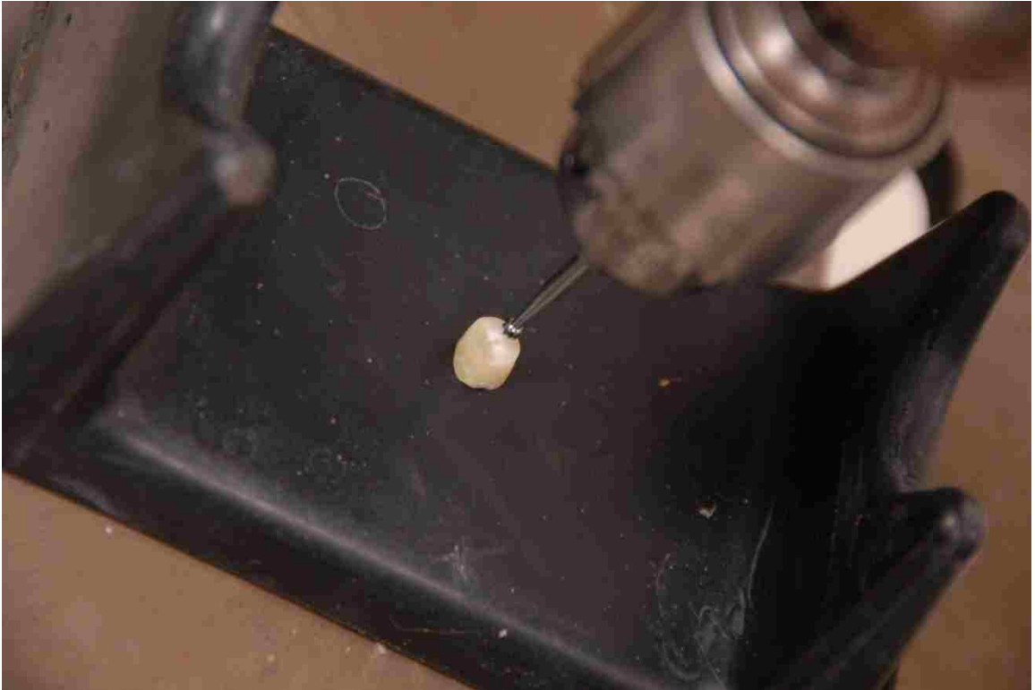
FIGURE 8. Close-up of ISO 025 bur in drill press and dentin specimen.
