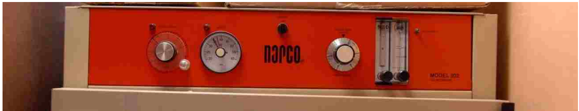
FIGURE 20. Incubator settings at either 37°C or 46°C with 5 percent CO 2 .
