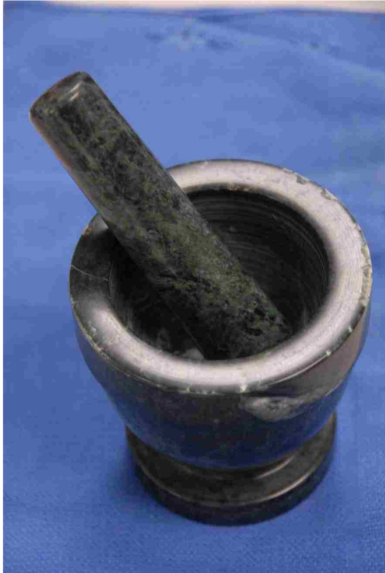
FIGURE 23. Mortar and pestle used in conjunction with liquid nitrogen to pulverize the dentin specimens.
