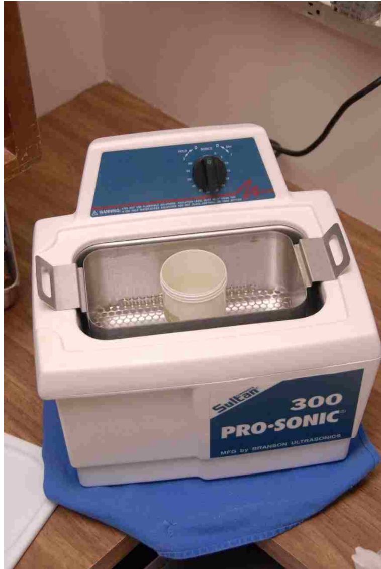
FIGURE 10. Ultrasonic unit used to aid in the removal of the smear layer.
