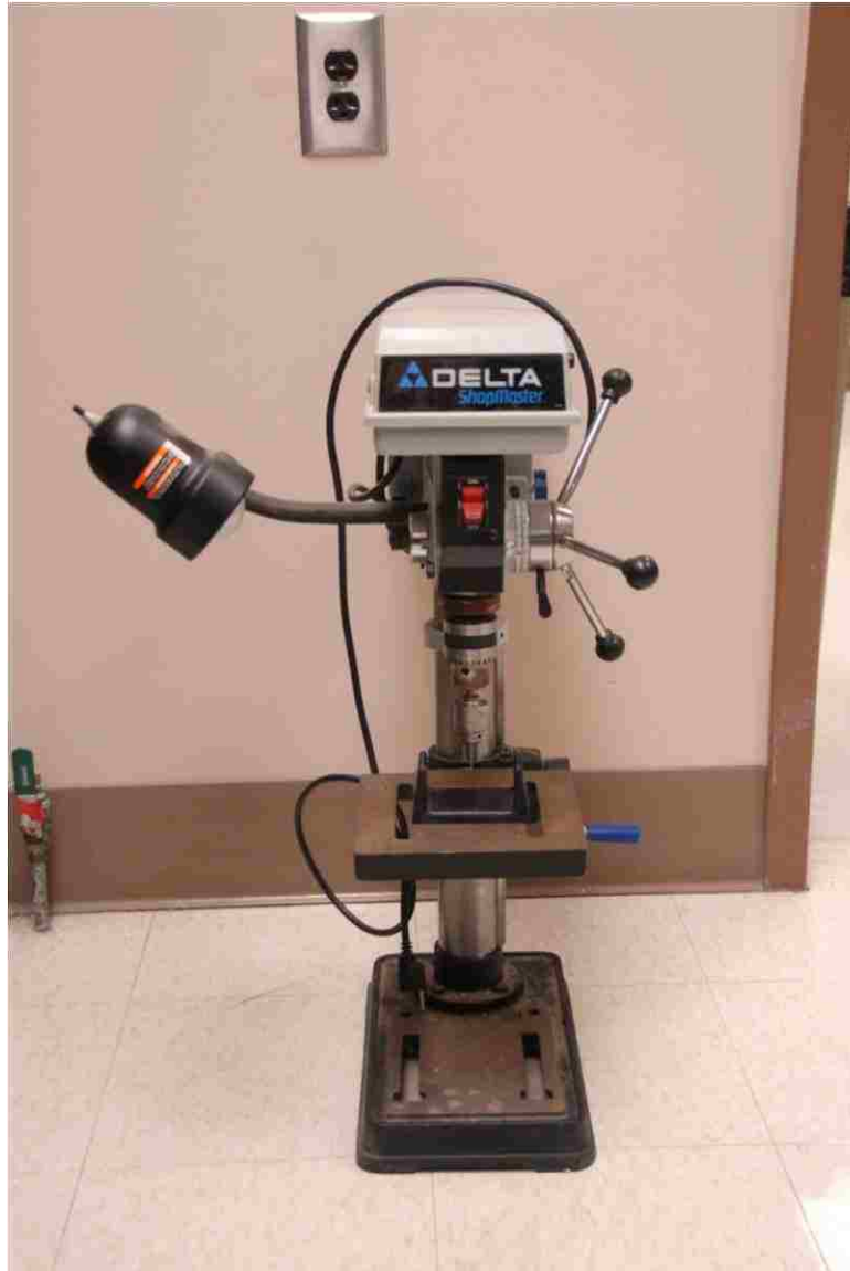
FIGURE 7. Heavy duty drill press used to prepare lumens in dentin specimens.
