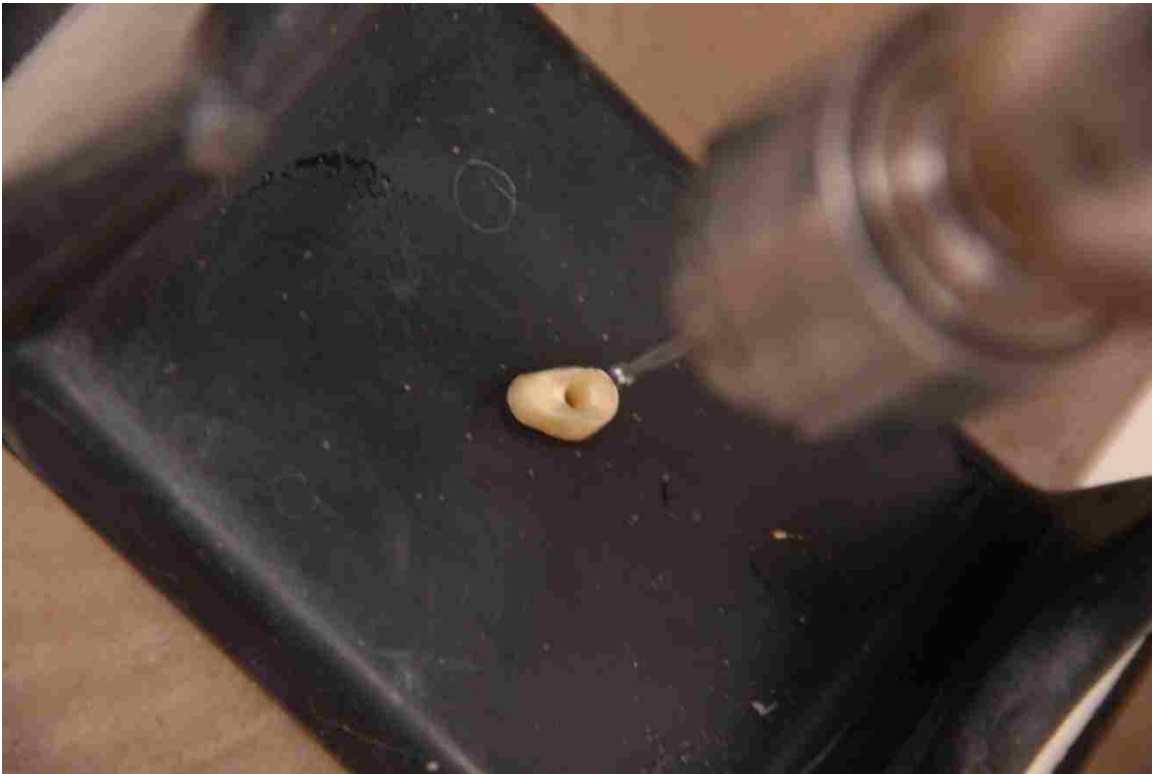
FIGURE 9. Close-up of 2.5-mm diameter lumen prepared in dentin specimen.
