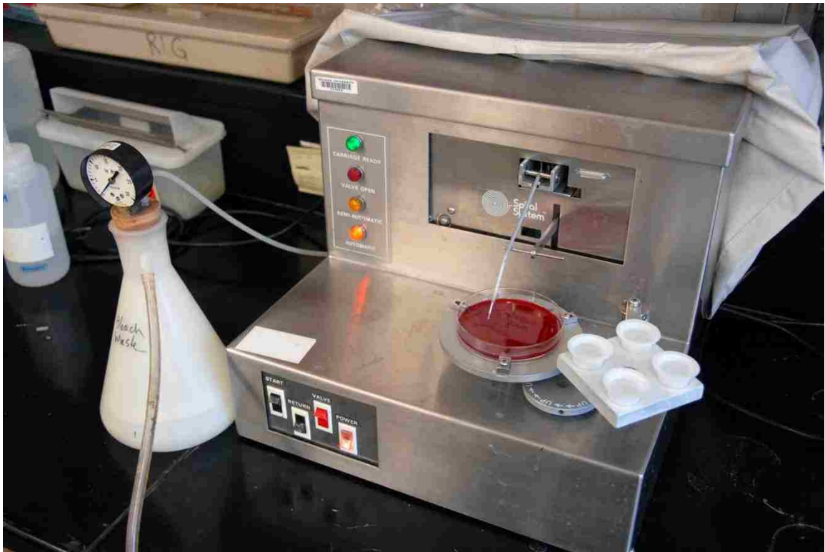
FIGURE 26. Spiral System used to spiral plate E. faecalis on the BHI agar plates.
