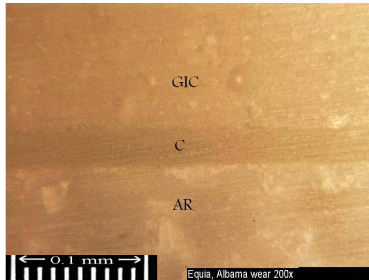
FIGURE 9. Cross-sectional micrograph of EQUIA specimen before three-body Alabama wear test. (Specimen 2) (GIC= glass ionomer; AR= acrylic resin; C= nano-filled resin coat)
