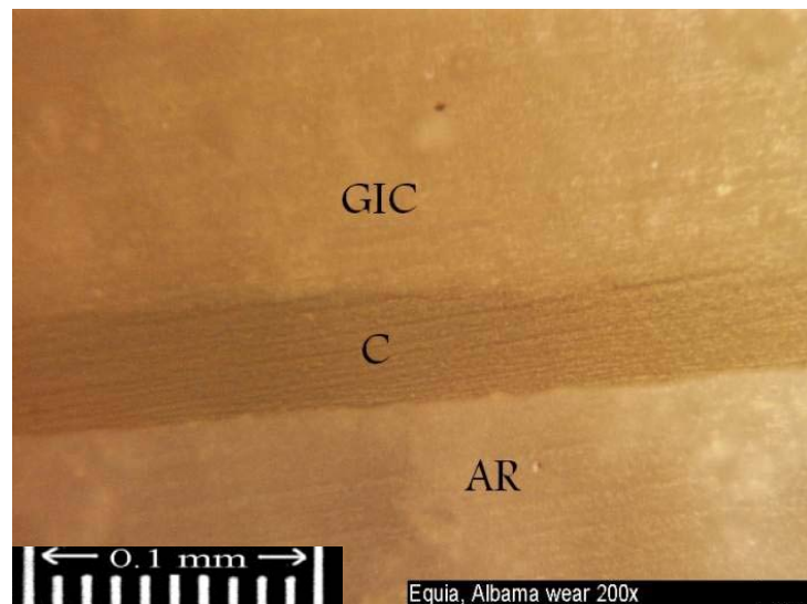
FIGURE 12. Cross-sectional micrograph of EQUIA specimen after three-body Alabama wear test. (Specimen 3) (GIC= glass ionomer; AR= acrylic resin; C = nano-filled resin coat)
