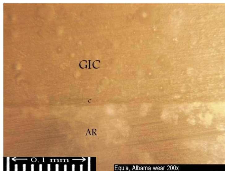
FIGURE 10. Cross-sectional micrograph of EQUIA specimen after three-body Alabama wear test. (Specimen 2) (GIC= glass ionomer; AR= acrylic resin; C= nano-filled resin coat)
