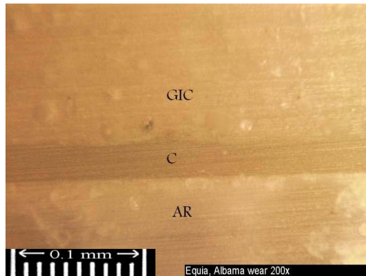
FIGURE 8. Cross-sectional micrograph of EQUIA specimen after three-body Alabama wear test. (Specimen 1) (GIC= glass ionomer; AR= acrylic resin; C= nano-filled resin coat)
