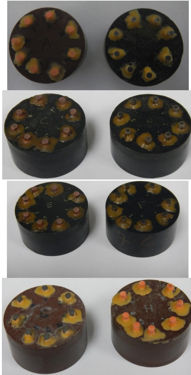
FIGURE 14. Visual comparison of Resilon to gutta-percha following bacterial exposure.
