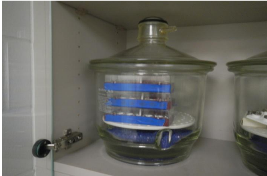
FIGURE 13. Samples placed in vacuum desiccator for 2 weeks prior to SEM and EDS analysis.
