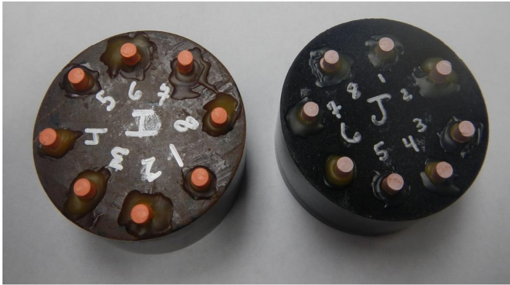
FIGURE 2. Samples mounted on ceramic discs with sticky wax.
