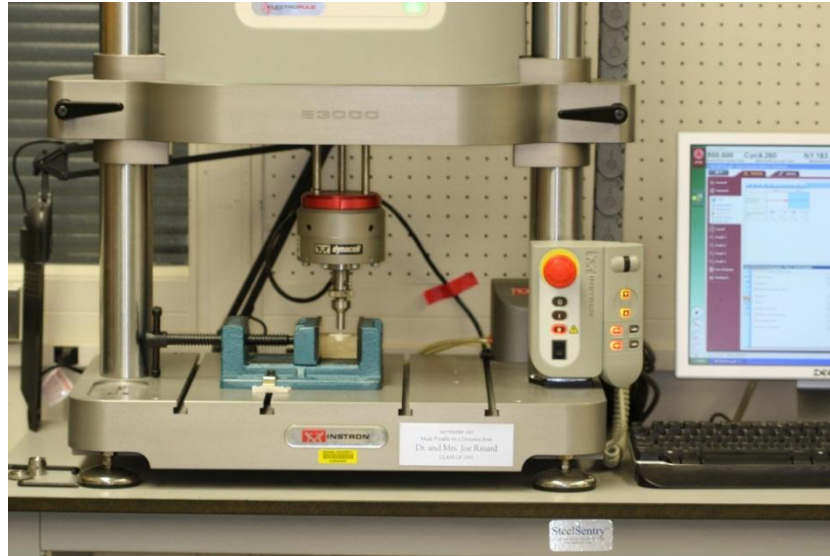
FIGURE 21. Illustration of mechanical cycling machine (Electropuls 3000, Instron).
