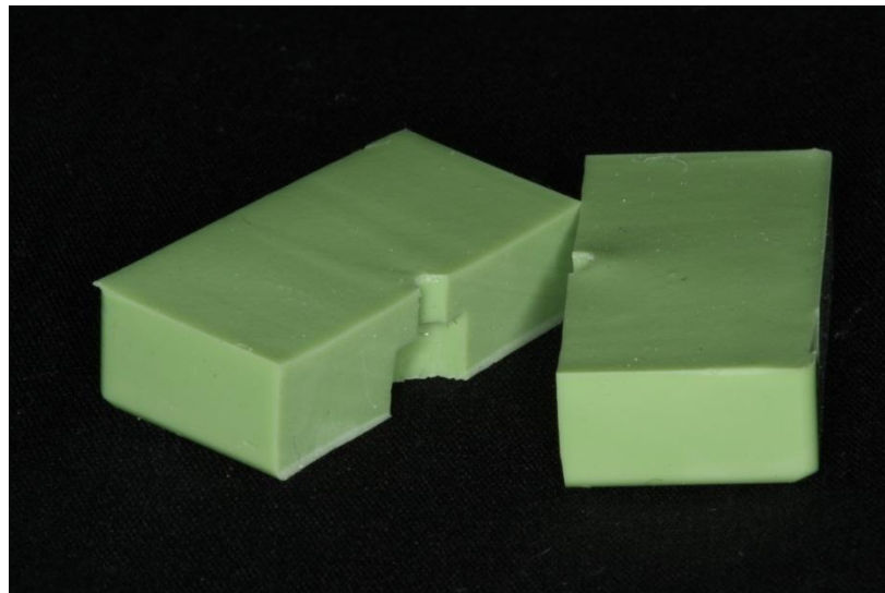
FIGURE 10. Illustration of a custom-made split silicone mold.
