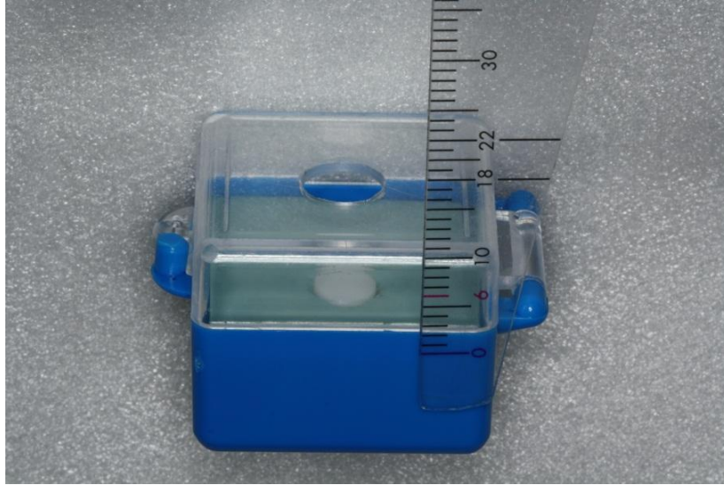
FIGURE 7. Illustration of customized plastic box to abrade Y-TZP as evenly as possible.
