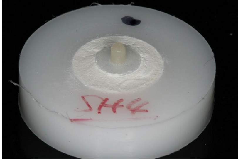
FIGURE 19. Illustration of the specimen embedded in the acrylic resin mold with type 4 stone.
