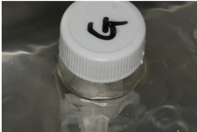
FIGURE 4. Illustration of cleaning of specimens in an ultrasonic bath containing acetone.
