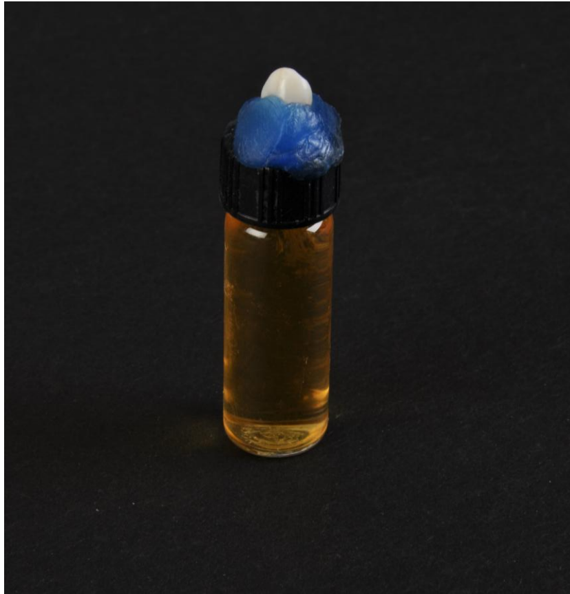
FIGURE 15. Photograph of assembled microbial leakage apparatus.
