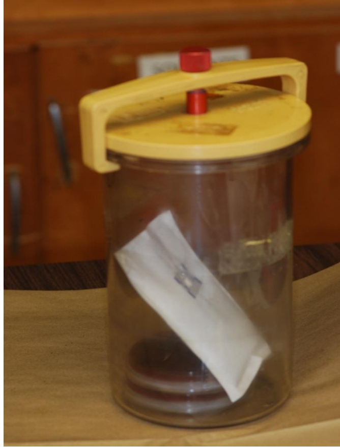
FIGURE 12. GasPack used to maintain anaerobic conditions during cultivation of Pg . After assembly the GasPack was placed in an incubator for 48 hours.
