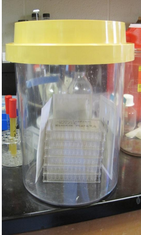
FIGURE 16. Microplates in GasPack container to maintain anaerobic conditions. GasPack container was sealed for 48 hours and incubated before spectrophotometer reading.
