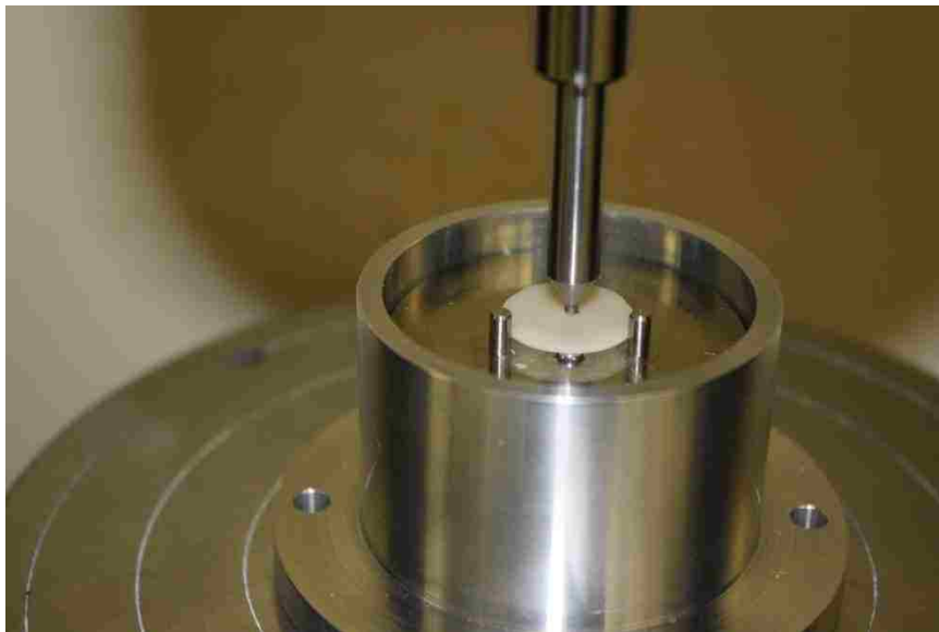
FIGURE 18. Illustration of ceramic specimen set up on a-three-ball jig and the position of a piston ready for loading
