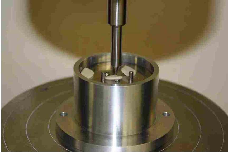
FIGURE 19. Illustration of ceramic specimen fracture after force loading
