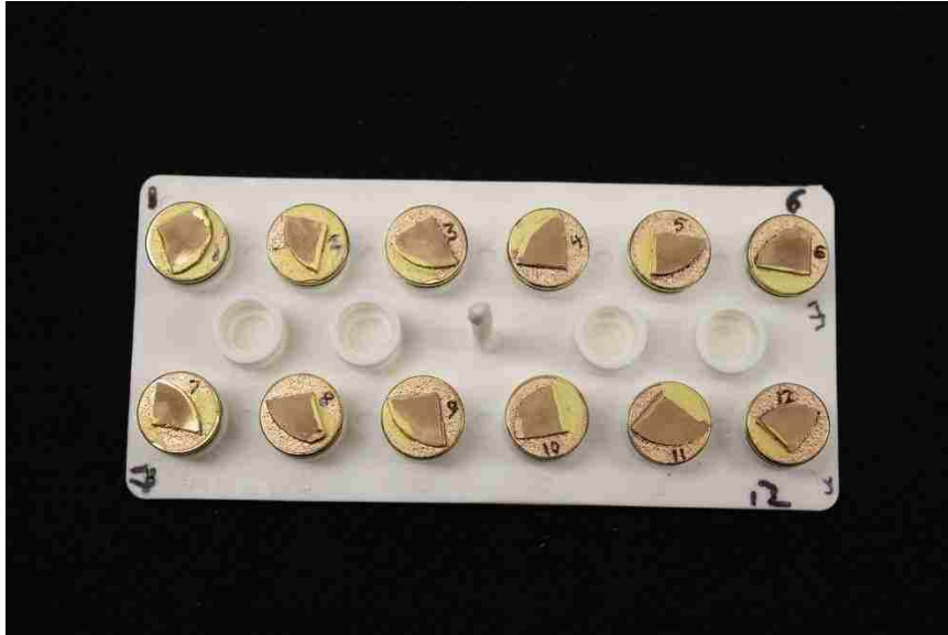
FIGURE 12. Illustration of specimens preparation for SEM
