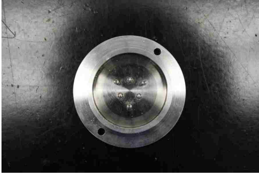
FIGURE 15. Illustration of a-three-ball-jig for biaxial flexural strength
