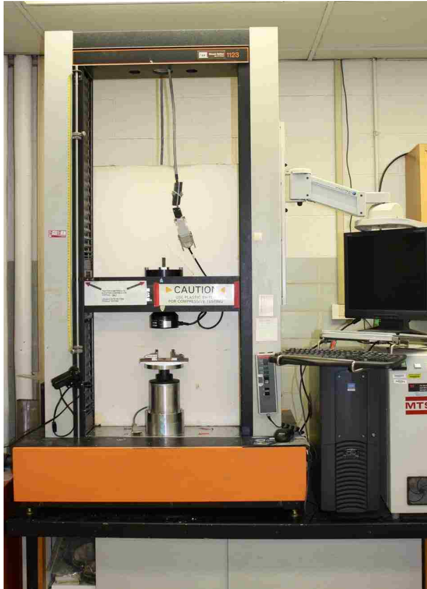
FIGURE 16. A universal testing machine (MTS Sintech ReNew 1123) used for biaxial flexural test
