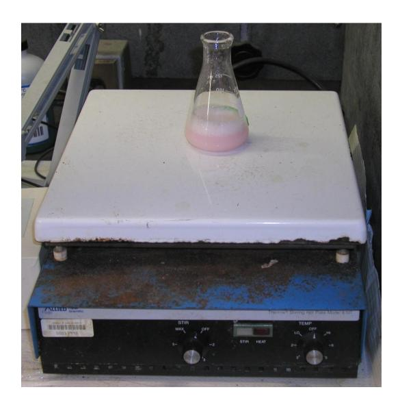
FIGURE 11. Stirring plate with Resilon emulsions to stabilize emulsion and evaporate chloroform.
