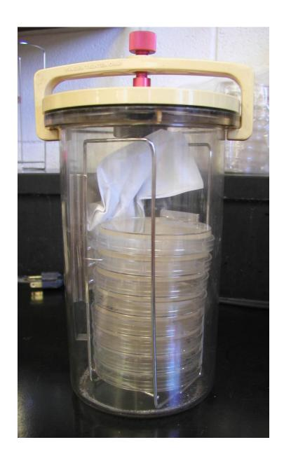
FIGURE 20. Anaerobic chamber for bacteria.
