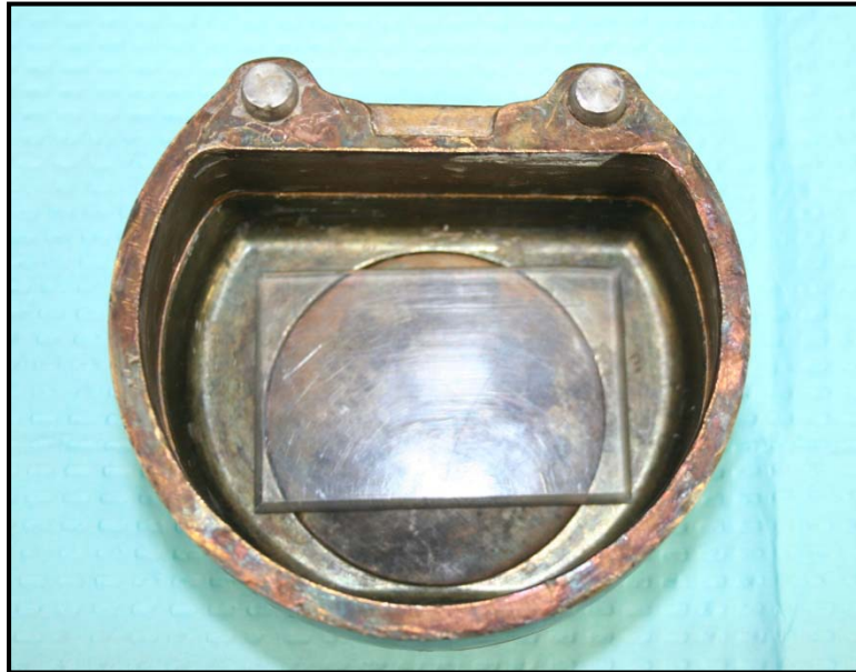
FIGURE 3. Image of denture flask and plastic mould used for sample fabrication.
