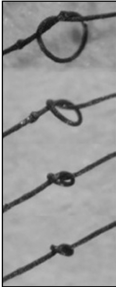
FIGURE 9. Micrograph taken from Vigolo et al 25 showing the exceptional flexibility of carbon nanotube based fiber (15 \mu m radius fiber).
