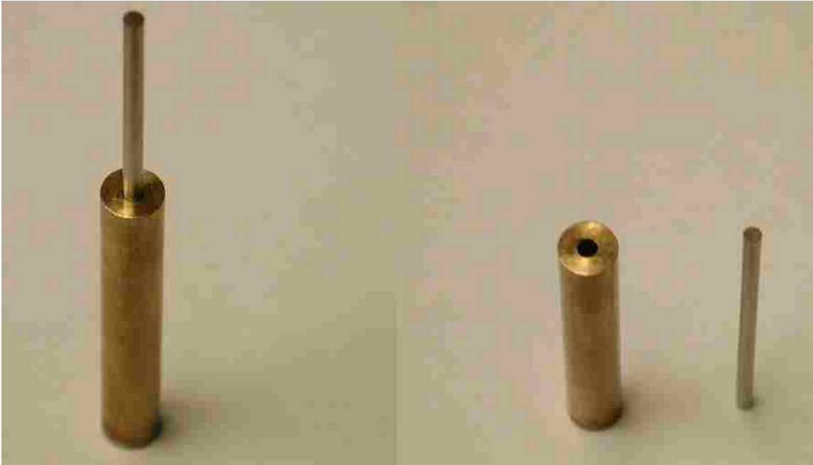
Figure 5. Alignment tool, as used for alignment (left) and with separated cylinders for specimen scanning (right).
