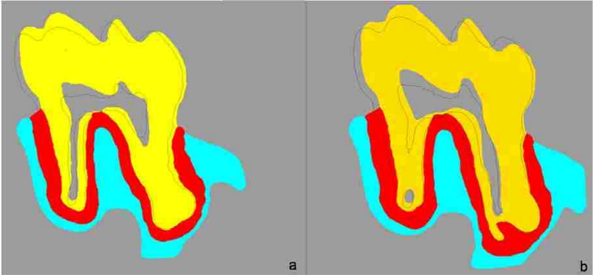
Figure 31. Static sections of the 3D FE model showing calculated initial (contour) and final (solid) positions of the teeth on the A , ERR analysis section plane and B , bone formation analysis section plane. Because the sections followed stress directions, the tooth has negligible out-of- plane movement. This is evidenced by little change observed in tooth and root shape between the initial and final positions in these planes.
