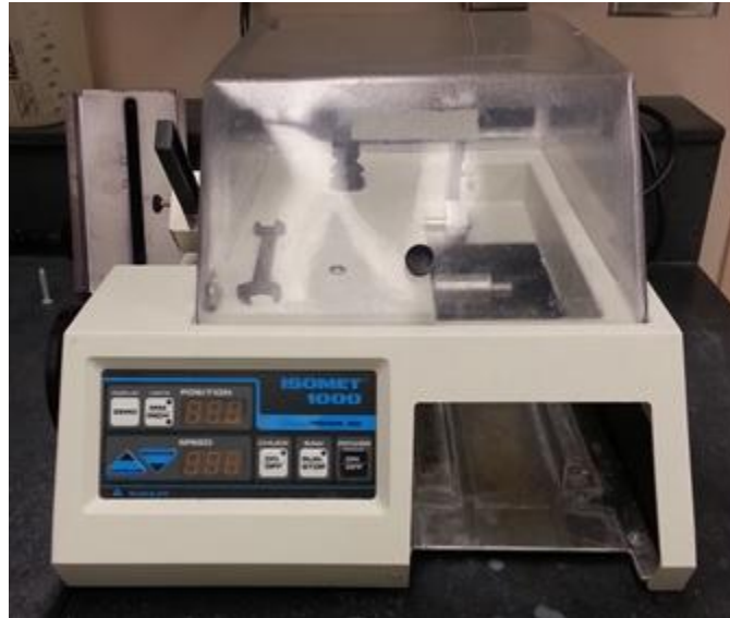
FIGURE 1. Isomet 1000, a cutting machine.
