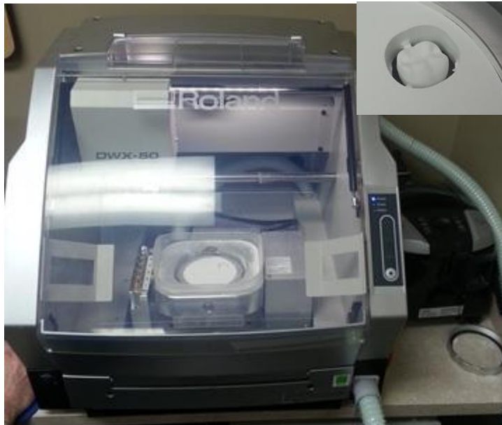
FIGURE 9. Roland CAD/CAM machine for zirconia.
