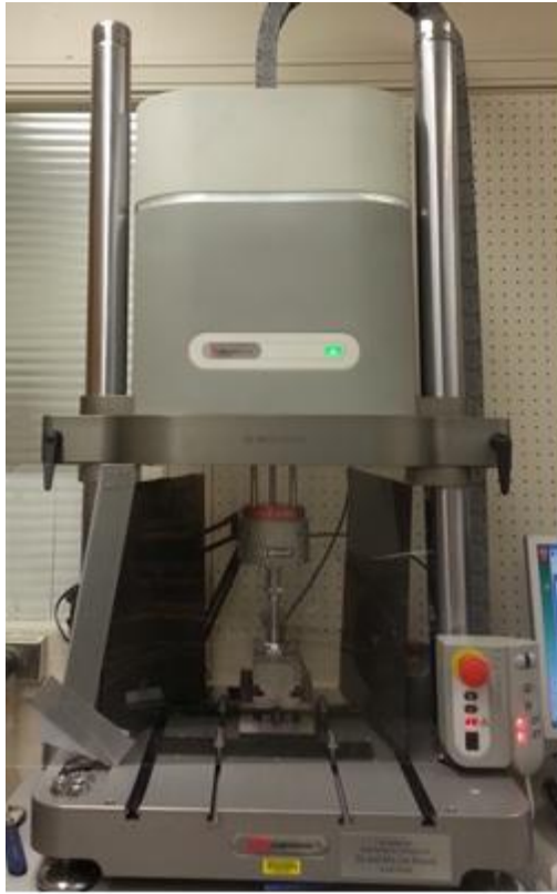
FIGURE 14. Instron E3000, loading machine.
