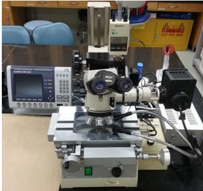
FIGURE 3. Nikon measuroscope used to measure and examine the notches.
