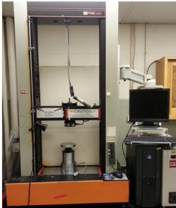
FIGURE 4. MTS Sintech 123, a loading machine.
