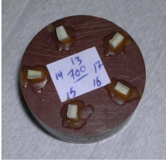
FIGURE 7. Photographs of polishing the simulated cavity wall of the specimens. Specimens were mounted on plastic blocks using sticky wax (a) and then ground and polished on a rotary machine (b).
