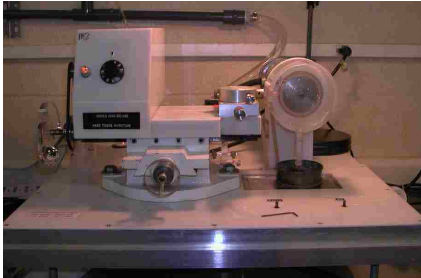
Figure 7 – Photograph of the hard tissue microtome for obtaining sections for TMR (top). A specimen glued on plastic rods before sectioning (b). A section examined using a stereomicroscope (c).
