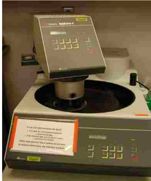
Figure 2 – Photographs of the steps of polishing the enamel slabs. The polishing machine (top), enamel slabs mounted on acrylic blocks using sticky wax (middle), and then ground and polished on the rotary part of the machine (bottom).
