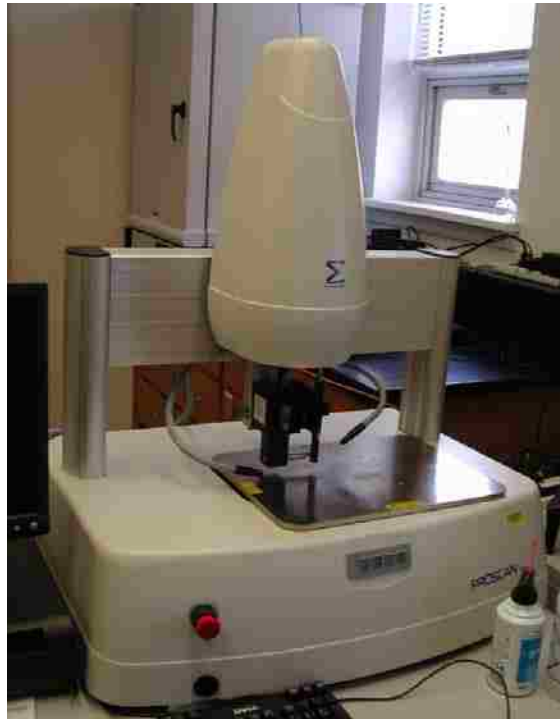
Figure 4 – A photograph of the optical profilometer used in the project (top) and a close-up photograph of the optical sensor with a specimen ready for scanning (bottom).
