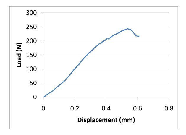
FIGURE 9. Chart showing a typical load-displacement curve from the pushout test.
