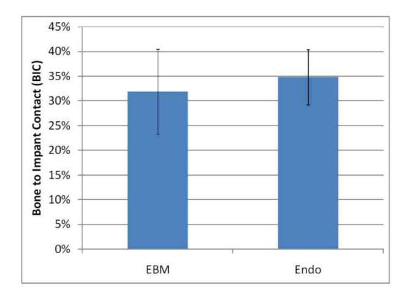
FIGURE 8. Chart showing the bone-to-implant contact (BIC) of EBM (Southern Methodist Univ.) and Endopore (Innova Corp.) implant.
