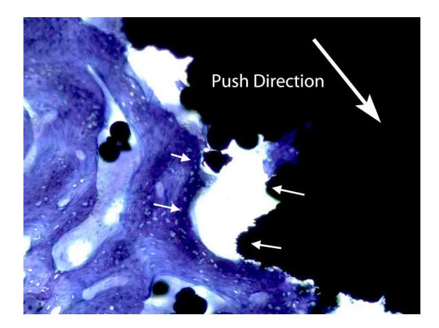
FIGURE 16. Histological picture of EBM (Southern Methodist Univ.) implant after pushout test. The direction of the pushout test is indicated by the large white arrow and the indentation of the implant on bone is indicated by the smaller white arrows. Note that part of the bone is attached to the implant at the area of fracture and part of the implant is still attached to bone as well.
