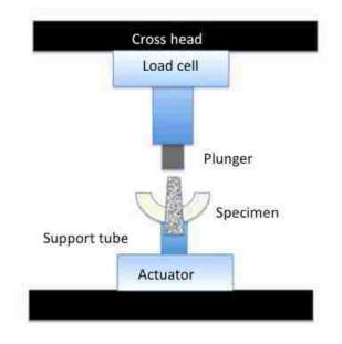
FIGURE 2. Schematic of a typical mechanical test fixture used in the pushout test. The support tube has an inner diameter greater than the diameter of the implant creating clearance.
