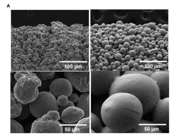
FIGURE 3. The surface of Endopore (Innova Corp.) (left) and EBM (Southern Methodist Univ.) <sup>31</sup> implants under SEM at X100 (top) and X1,000 (bottom).
