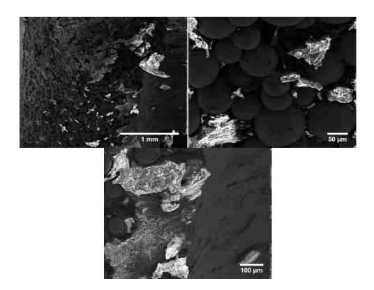
FIGURE 12. SEM Images of Endopore (Innova Corp.) implant surface after fracturing the bone at the implant bone junction: X50 (top left); X200 (bottom) shows the implant on the left and bone on the right; and at X350 (top right) bone pieces can be seen between the titanium implant beads.
