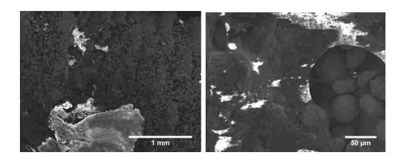
FIGURE 14. SEM images of EBM (Southern Methodist Univ.) implants after bone removal at the implant bone interface: At X50 (left), and more so at X500<sup>31</sup>, smooth areas appear on the implant surface where beads had been pulled away with the bone.
