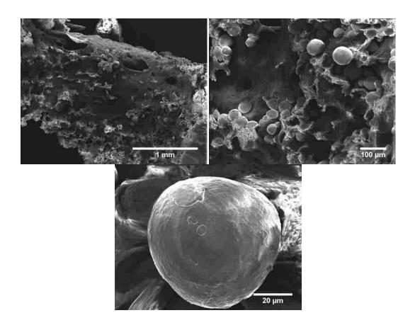
FIGURE 15. SEM images of the fractured bone surface apposing the EBM (Southern Methodist Univ.) implant. At X50 (top left) and X200 (top right) many titanium beads are attached to the bone surface. At X1500 (bottom) a fractured bead left on the bone is visible. The original attaching point can be seen on the upper left of the bead.
