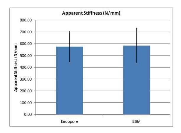
FIGURE 11. Chart showing the apparent shear stiffness from Endopore (Innova Corp.) and EBM (Southern Methodist Univ.) implants.
