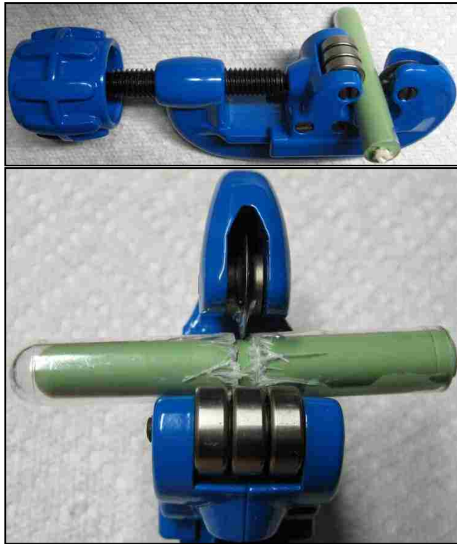
FIGURE 67. Plastic test tubes scored with plumbing pipe cutting device and separated from impression material.
