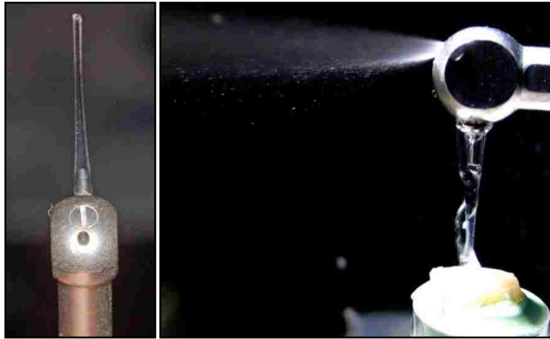
FIGURE 58. Exhaust vent of the Canal CleanMax.
