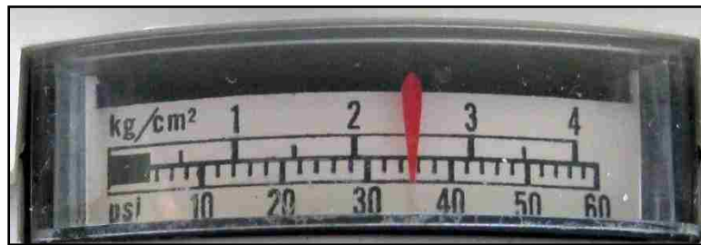
FIGURE 63. Adjusting dental unit to deliver 35 lbs per square inch of compressed air to high speed handpiece prior to connection of Canal CleanMax.
