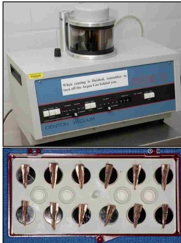
FIGURE 73. Specimens sputter-coated with gold-palladium. 333, 334
