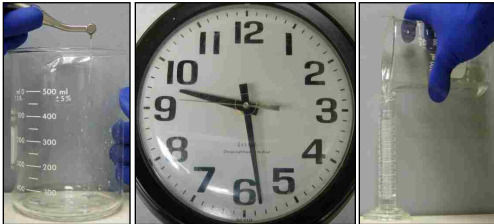
FIGURE 66. Determination of volume of sterile saline delivered from Canal CleanMax over 30 seconds.
