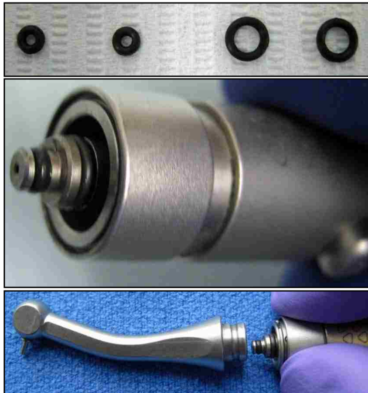
FIGURE 61. Replacement of O-rings of Canal CleanMax handpiece.
