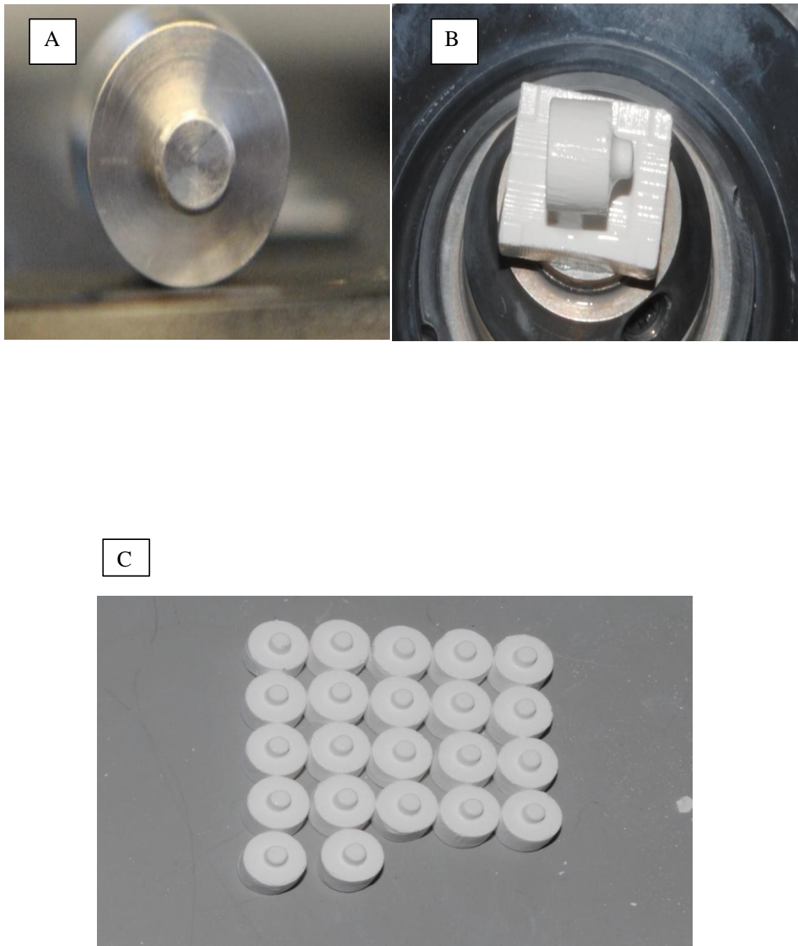
FIGURE 4. Zirconia sliders fabrication using CAD/CAM machine. A) Metal pattern prepared to be scanned by the CAD/CAM machine. B) The zirconia samples milled by the machine according to the scanned metal pattern. C) Zirconia specimens ready to be sintered.
