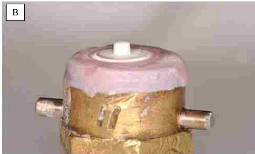
FIGURE 7. A) Schematic representation of zirconia slider showing the shape and dimensions of the slider. B) A mounted slider specimen with the slider tip extending above the mounting acrylic.
