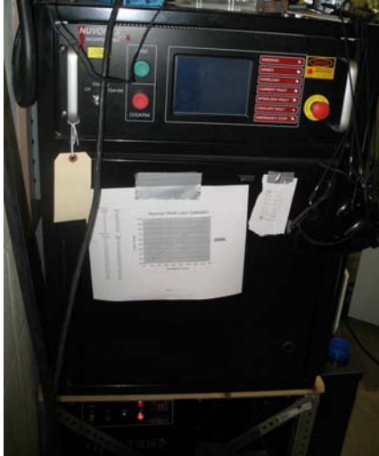
Figure 1. 1.0 KW Nuvonyx Diode Laser (808 nm wavelength)
