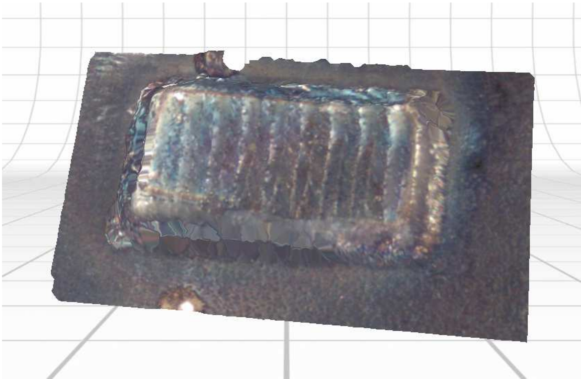
Figure 29. The part is deposited by Titanium powder
