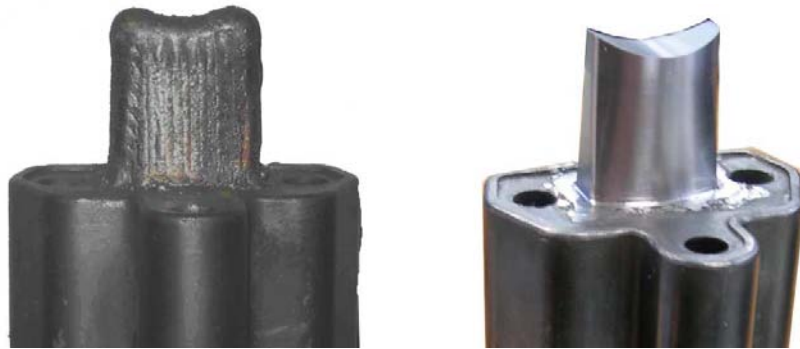
Figure 1. The die after repaired by laser deposition and machined by CNC
