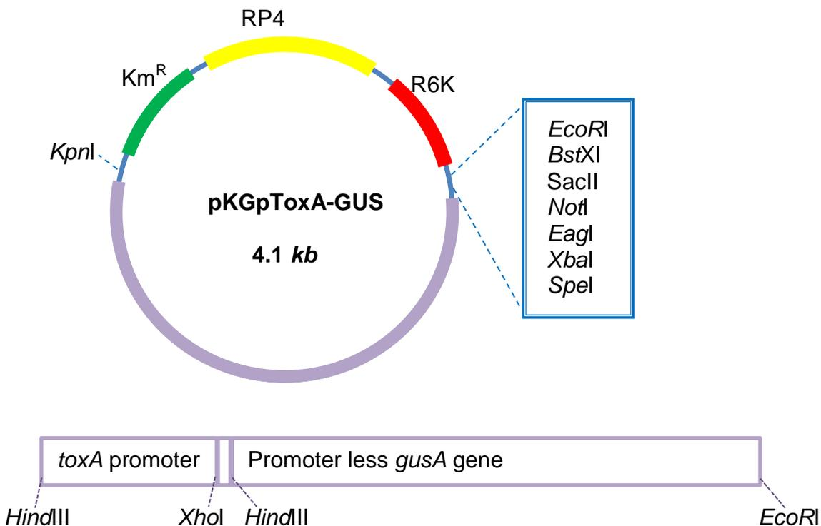
Figure 3.1. Construction of the newly generated vector pKGpToxA-GUS vector. The *toxA* promoter and promoter less *gusA* gene was inserted into the pKNOCK-Gm vector at *KpnI* and *SpeI* sites. pKGpToxA-GUS has Km<sup>R</sup> gene, RP4 and R6K origins, which give this vector Km resistance, conjugative and suicide properties.
