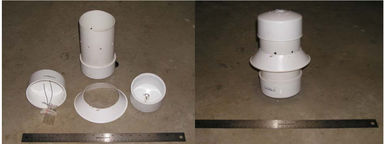
Figure 2.5. Pitfall trap viewed disassembled (left) and assembled (right) used to catch root feeding insects.
