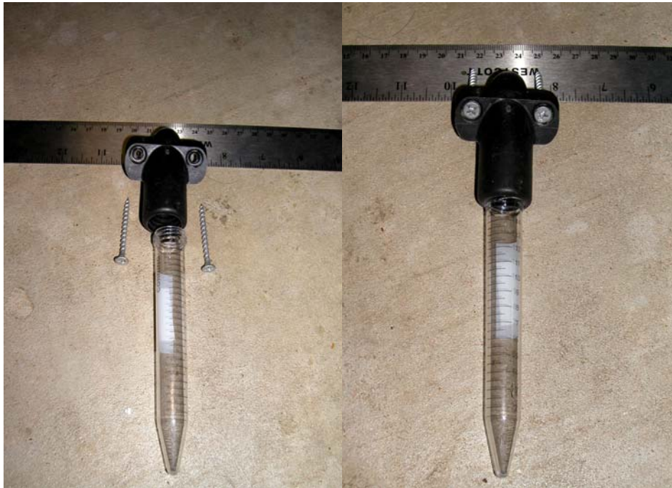
Figure 2.6. Resin sampler disassembled (left) and assembled (right) with polyethylene terephthalate centrifuge tube.
