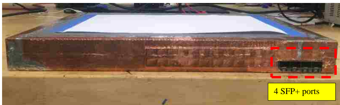
Figure 5.2. EUT 1 front view showing the ports for the four optical modules
