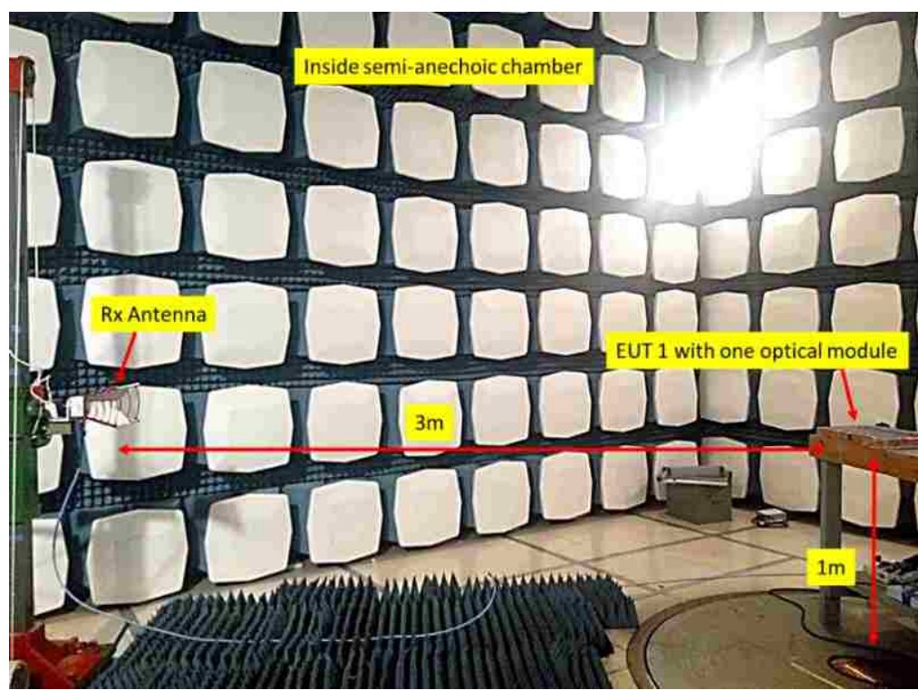
Figure 7.4. Actual photo of the setup inside the semi-anechoic chamber for E field measurement of one optical module in EUT 1.
