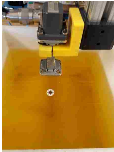
Figure 6.17. Embedded tag measurement setup for tag embedded 0 cm in oil.
