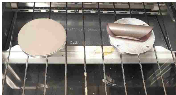
Figure 5.15. Sintered prints. Left: photo paper. Right: Mitsubishi paper.
