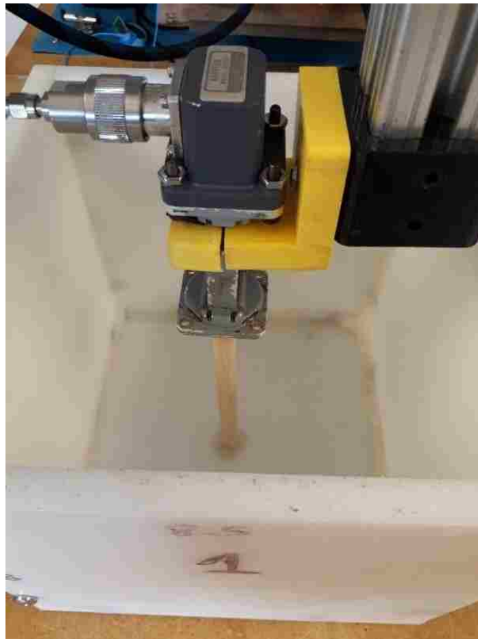
Figure 6.16. Embedded tag measurement setup.
