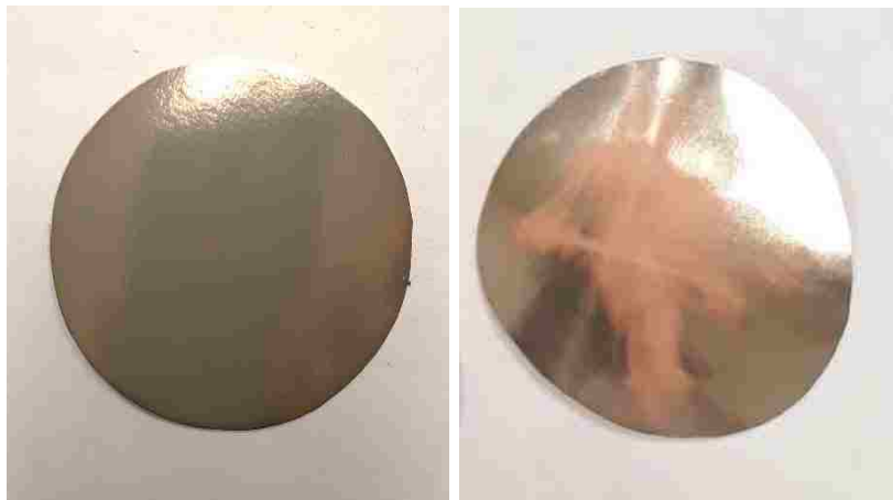
Figure 5.13. Effect of handling samples. Left: un-smearred. Right: Smearred.
