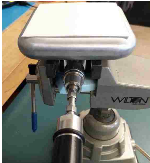
Figure 5.1. Setup for measurement of dielectric properties of paper.
