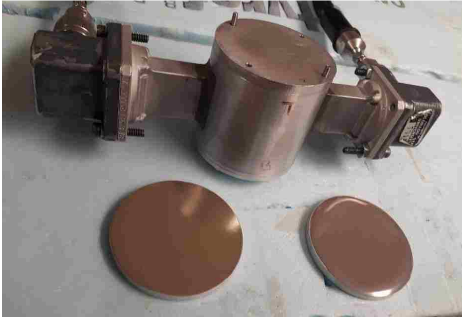
Figure 5.11. Measurement setup for conductivity measurements.
