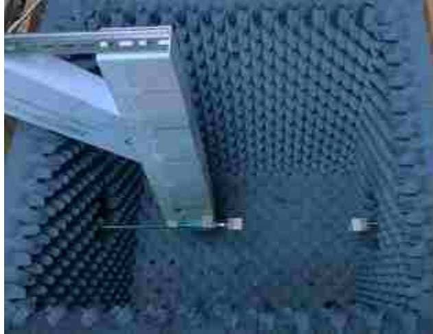
Figure 2.15. Test setup for determining the power transfer between two like antennas.
