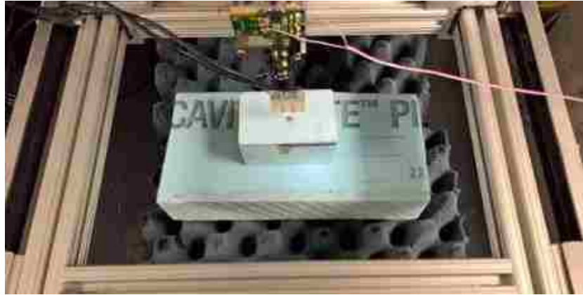
Figure 2.17. Designed antenna raster scanning over a small area.
