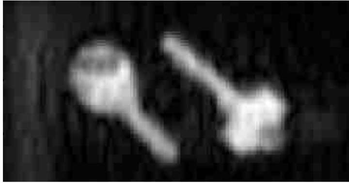
Figure 3.13. 2D image of both keys covered with a 4 mm sheet of rubber.
