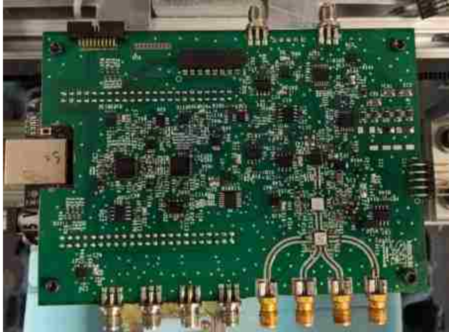
Figure 2.29. Fabricated controller board.
