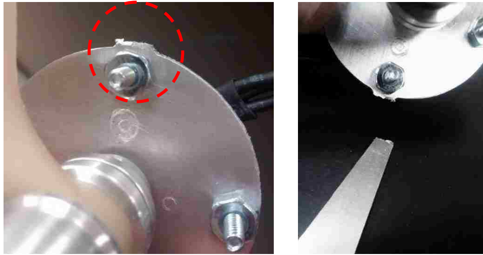
Figure 4.8. 0.050-in Beam Torsion Failure
