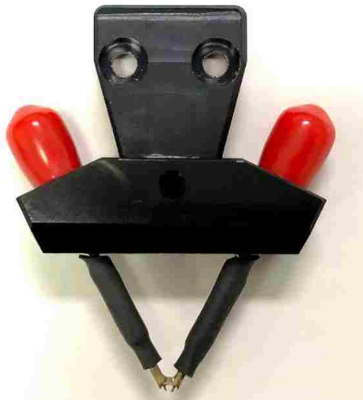
Figure 4.7. Differential probe (D-probe).
