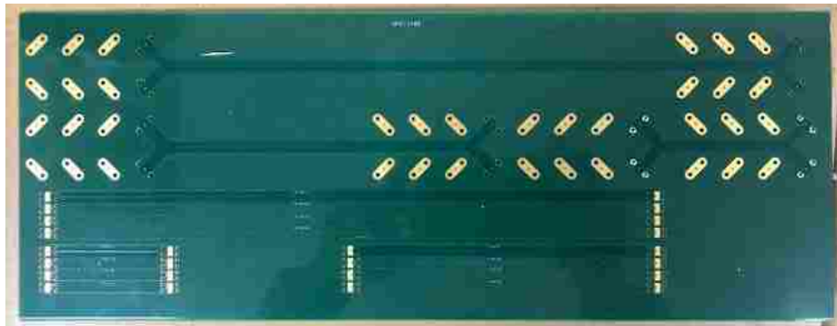
Figure 3.10. 0.5 mm pitch probe lunch pattern testing board.
