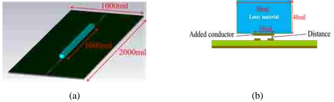
Figure 3.3. Proposed broadband CM suppression filter: (a) 3D view (b) cross section view.
