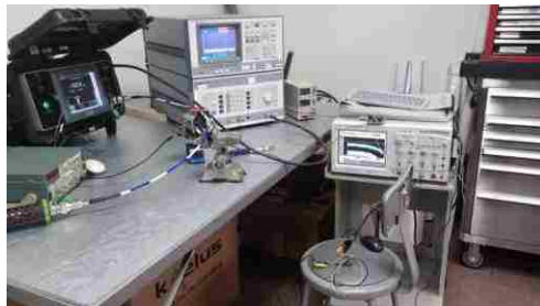
Figure 2.7. Measurement set-up of the vibration method.
