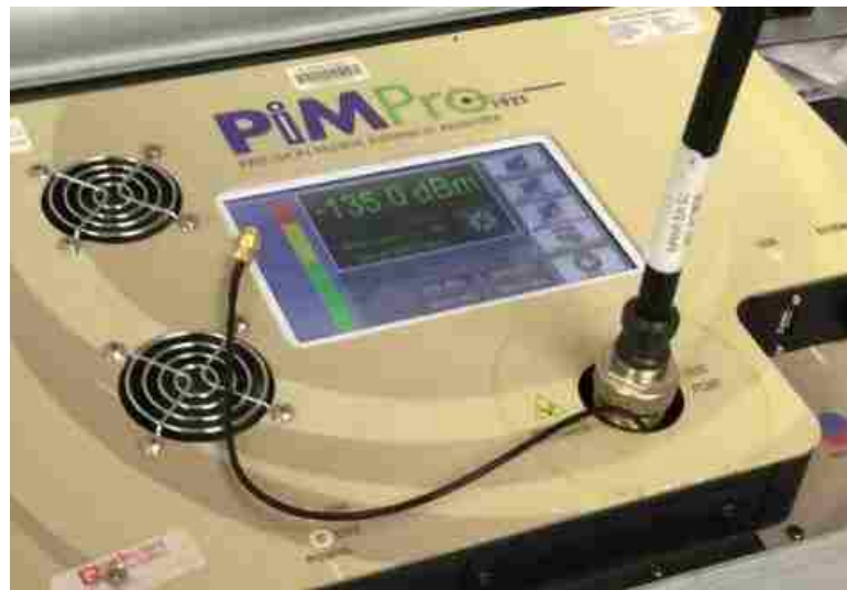
Figure 3.31. Modified analyzer with coax probe added for Rx (PIM) signal output.
