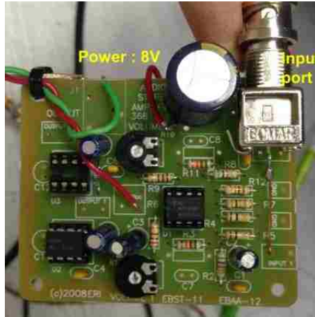
Figure 2.5. Audio amplifier for amplifying RF output of PIM tester.
