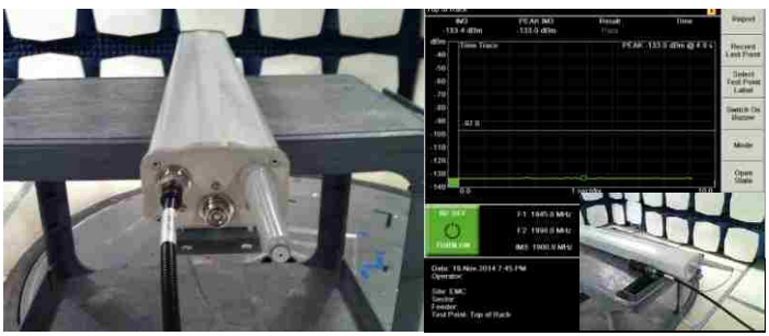
Figure 2.23. Antenna PIM level measurement set-up.
