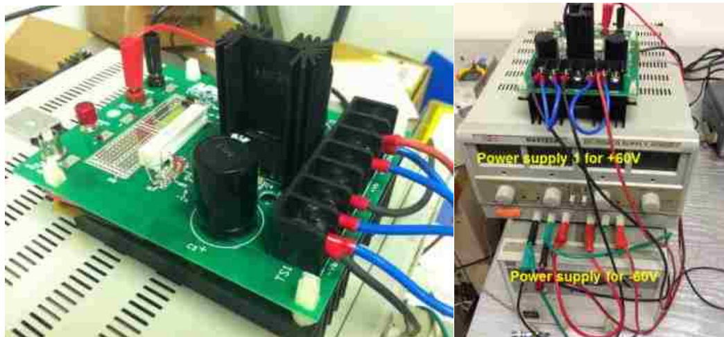
Figure 2.17. Apex MP118 evaluation kit to drive the transducer.
