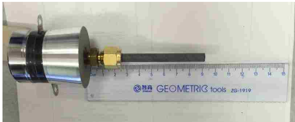
Figure 4.8. Ultrasonic transducer with ceramic rod structure
