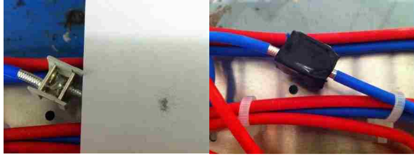
Figure 2.28. PIM source II: metal debris.
