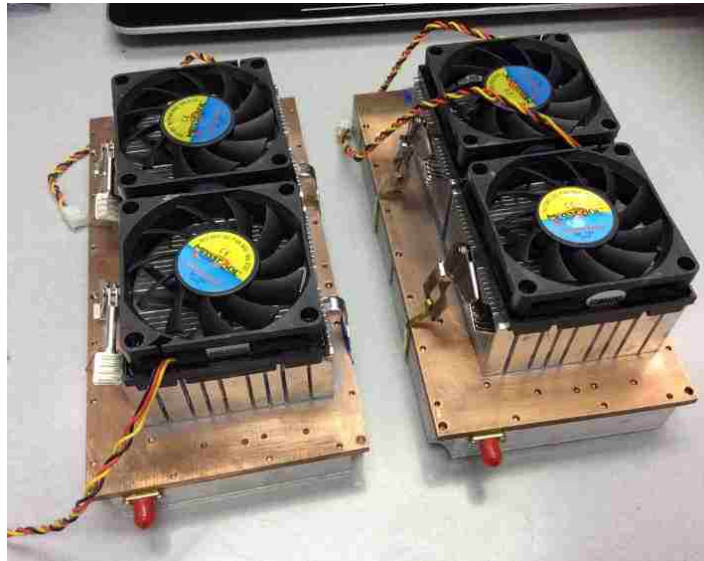
Figure 3.27. Two power amplifier purchased for the self-made PIM analyzer.
