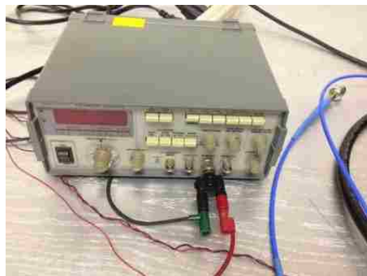
Figure 2.15. Signal generator to drive the speaker to operation frequency.
