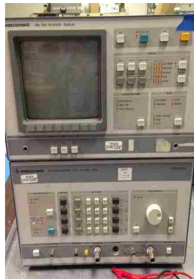
Figure 2.4. Rohde & Schwarz Spectrum Analyzer equipped with video output.
