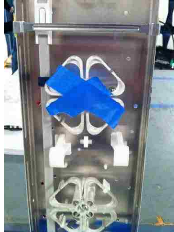
Figure 2.25. Small ferrite piece attached to the center of dipole antenna.
