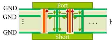
Figure 4.1. IC interconnection inductance extraction in the PCB.
