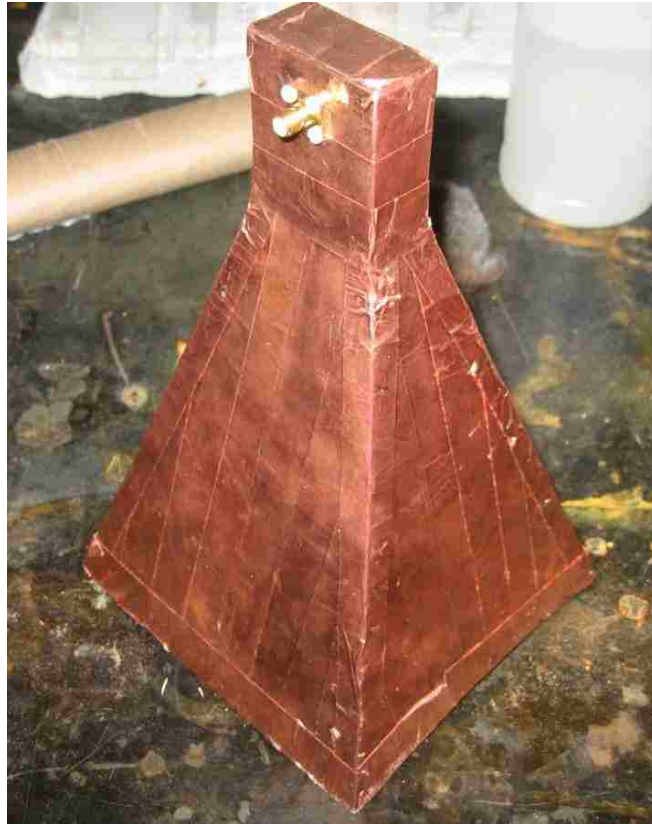
Figure 3.16. Filled horn antenna for measuring FSS embedded in concrete column.
