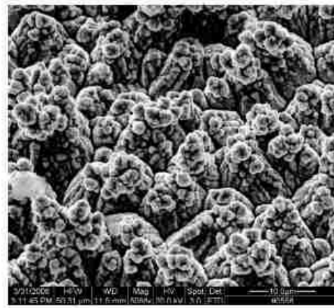
Figure 2.6 Copper foil surface SEM photograph [3]
