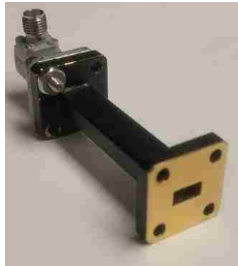
Figure 2.1: Standard linearly polarized open-ended rectangular waveguide probe.
