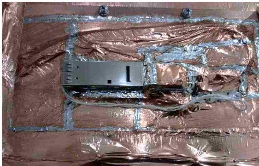
Figure 3.19 Close View of the Cage Area in the Measurement Setup
