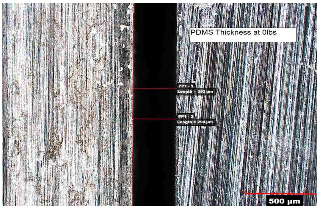
Figure C. Compressed thickness at various applied load (a) 0 lbs.
