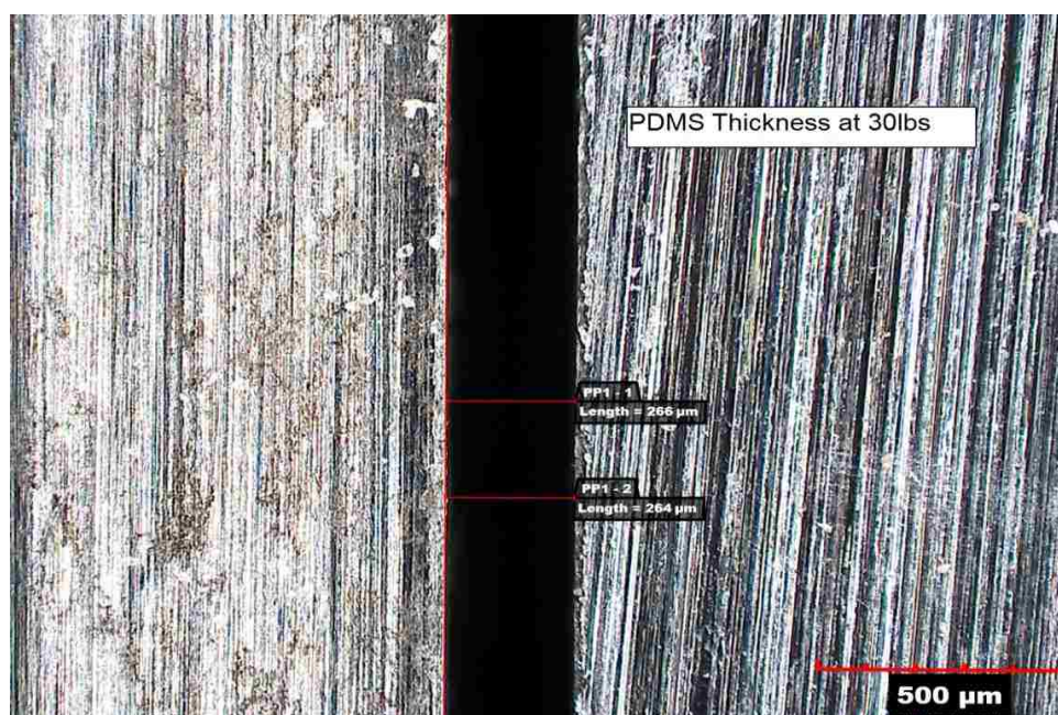
Figure C. Compressed thickness at various applied load (d) 30 lbs (cont.).
