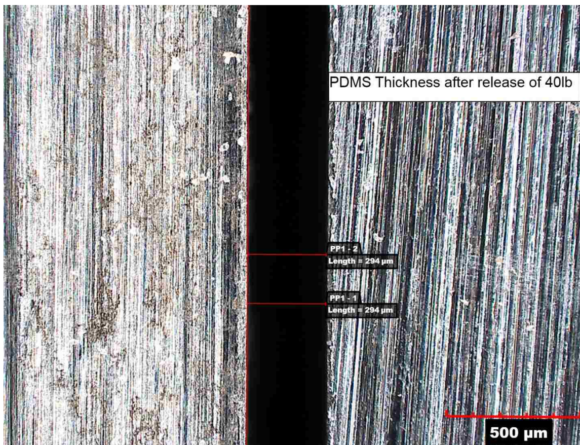
Figure. 4.7. Optical microscope images of PDMS elastomer (a) taken during compression at 0 lb, (b) taken during compression at 40 lbs, (c) taken during release of 40 (cont.).
