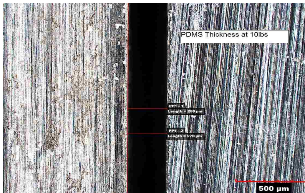
Figure C. Compressed thickness at various applied load (b) 10 lbs (cont.).
