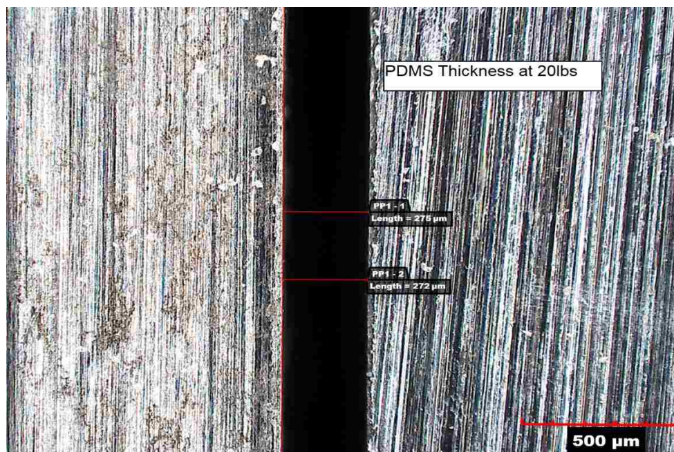
Figure C. Compressed thickness at various applied load (c) 20 lbs (cont.).
