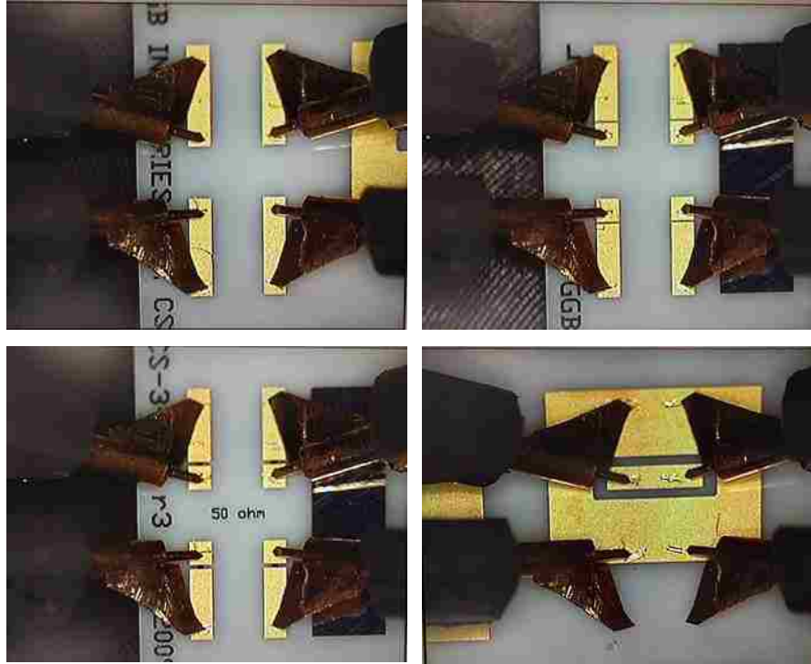
Figure 5.15. Probe calibration on CS3-1000 substrate. Short (top left), Open (top right), load (bottom left), thru (bottom right)
