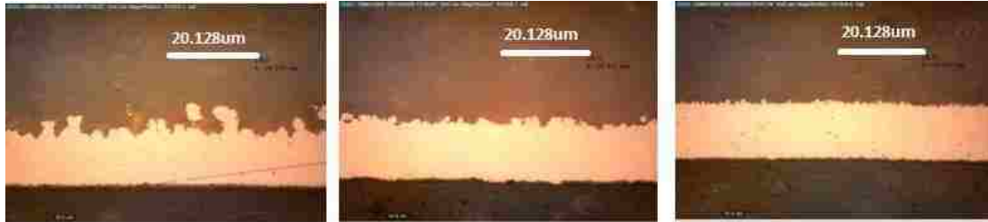
Figure 1.2. Optical microscopic images of roughness. From left to right: STD (standard), VLP (very low profile), HVLP (hyper very low profile)
