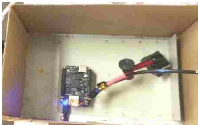
Figure 2.3. DUT placed inside an opaque screen with TLP injection probe.
