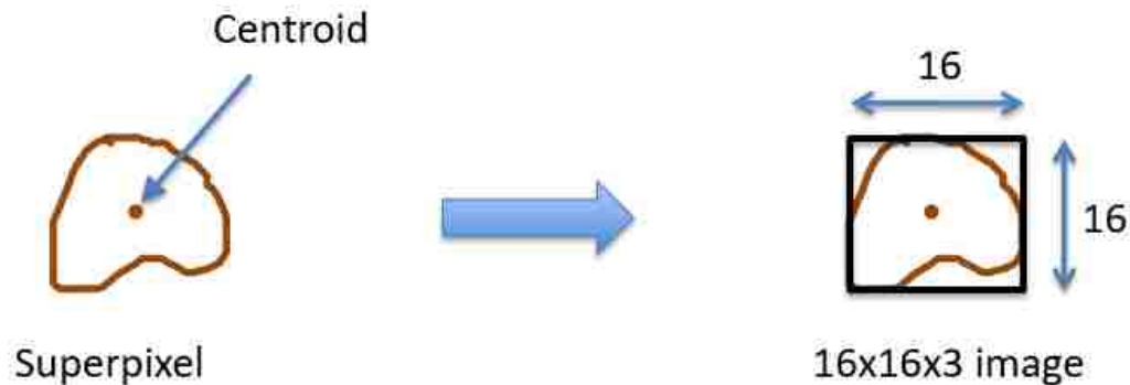
Figure 3.2 Generation of 16 \times 16 \times 3 RGB image from superpixel
