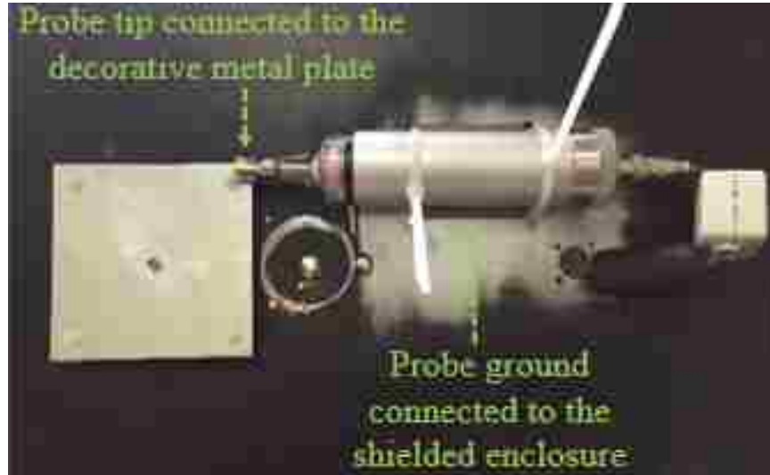
Figure 2. 1000:1 high voltage Tektronix probe is used for measuring the decorative floating metal voltage. Gasket is used at the tip of the high voltage probe and the decorative metal to ensure electrical contact between the two surfaces.
