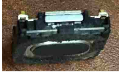
Figure 5. Audio transducer that sits below the earpiecemesh.
