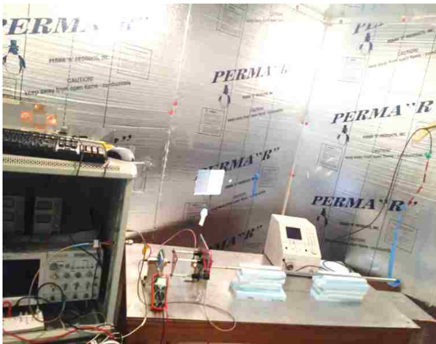
Figure 1. Test setup showing the rod, arc length measurement, oscilloscope in a shielded enclosure and the high voltage supply inside a climate chamber.
