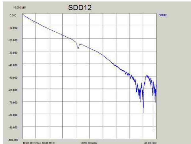
Figure 3.7. Measured differential insertion loss with a dip effect by glass weave
