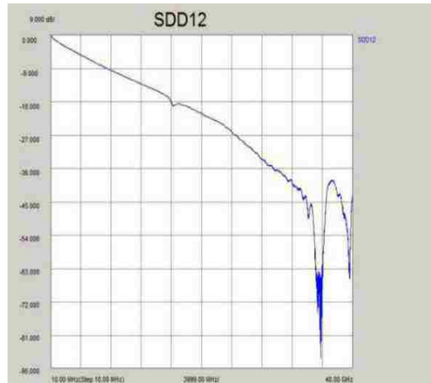
Figure 5.7. Differential insertion loss for the 12 inches trace
