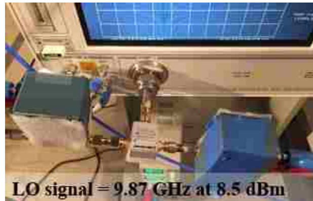
Figure 5.8. 20 GHz VNA signal output connected the splitter and the amplifiers. The output of the amplifiers is connected to the local oscillator port on the mixer.
